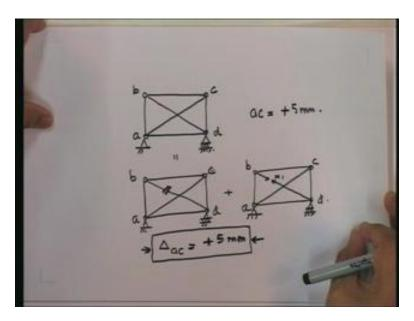
Therefore, we have this situation that member ac is longer. What is going to happen? You have this structure; no loading on it at all, this is a, b, c, d. The only thing that we are trying to find out over here is that ac actually has a positive lack of fit. In other words, what we have is, member ac is 5 millimeters longer than it should be. I can look at this problem in this manner that in the base structure....
