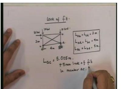
equal to length of cd is equal to 3 meters; length of ad is equal to length of bc is equal to 4 meters; length of ac is equal to length of bd is equal to 5 meters.
