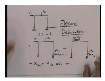
I am not going to solve this problem today because during the next few weeks, we are going to solve enough number of problems; I want to just introduce the concept to you. Let us say that I have gravity loading and some wind loading on this structure. What is the redundancy of this structure? If you look at it, you will get static indeterminacy is 1.
