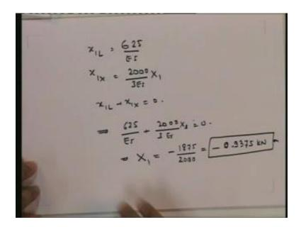
What is the compatibility condition going to give us?  $X_{1L}$  is equal to 625 upon EI,  $X_{1X}$  is equal to 2000 upon 3EI into  $X_1$ , compatibility condition  $x_{1L}$  plus  $x_{1X}$  is equal to 0. This implies that 625 by EI plus 2000 upon 3EI into  $X_1$  is equal to 0. This implies that  $X_1$  is equal to minus 1875 upon 2000, which is equal to minus 0.9375 Kilonewtons. Once I have this, note something very interesting. How do I get the bending moment diagram for the entire thing?
