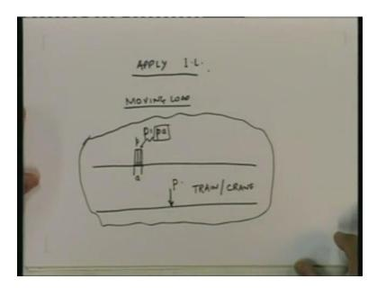
Where do we apply influence line? It is obviously moving load. What kind of moving load can we have? We can have something like this that over some a we have some load intensity which is given uniformed intensity  $P_a$  so that total load is P into a. When does this kind of a thing happen? This happens when you have a truck or a car traveling over a bridge. There is an area over which the load is distributed.
