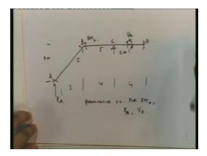
In this problem this is my e point which is 2 meters identical. This is the same problem in fact for M I I I this is 3, this is 4, this is 4 A B C D and I ask you to find out  $R_A$ , the sheer  $V_E$  and the bending moment at B, quantitative influence line for bending moment at B R at a and V at E. You find these out I have already done this I will give you the answers for your computation.
