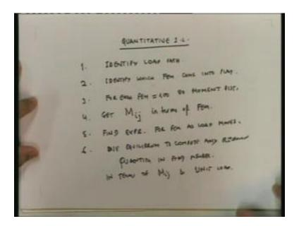
Steps for quantitative influence lines: first identify load path, identify which fixed end moments come into play. When you know the load path you know exactly from which fixed end moments are going to be non zero as the load moves from which ever point to which ever point we wanted to move. Identify which come into play. For each FEM equal to 100 do moment distribution. As many number of points at which you develop fixed end moments you are going to get that many moments to distribute.
