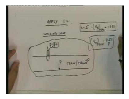
For maximum value of  $V_E$  we need to put it just to the left. So, x equal to 2 minus is  $V_E$  max and the value for a unit load is equal to plus point 511. When we have this, for this load, this moving we know what the maximum  $V_E$  is going to be, we know where the load has to be applied, it has to be applied at this point and once we apply the load at this point you can do analysis and you can get  $V_E$  max is equal to 0.51 P.
