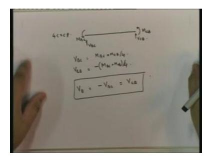
If the load is between 4 and 8 then BC becomes  $M_{BC}$   $M_{CB}$  the load is no longer there. We have  $V_{BC}$  and  $V_{CB}$  and we see that  $V_{BC}$  is equal to  $M_{BC}$  plus  $M_{CB}$  by 4 and  $V_{CB}$  is equal to minus of  $M_{BC}$  plus  $M_{CB}$  by 4. If we look at it then  $V_{E}$  is equal to minus BC or which is also equal to  $V_{CB}$ . This is minus and this is minus (Refer Slide Time: 22:23). Now let us look at how to compute. What we do is we compute.
