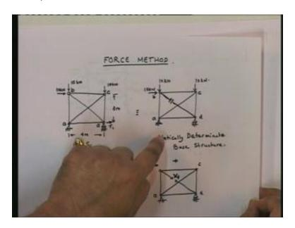
These are the forces that I found out for this particular structure which is the statically determinate base structure. I have found out the forces in all the members. What is the next step? The next step is actually to find out the deformations in all the members. What are the
