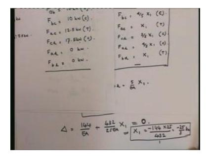
This in essence is the force method and I hope that with this simple illustration I have been able to illustrate the basic concept of the force method as applied to a single static indeterminacy truss. Thank you.
