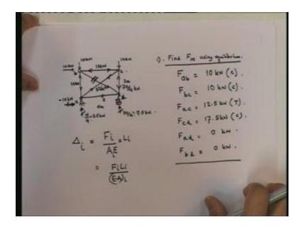
This is the real structure, I am trying to find out the displacement at this point because of all these forces. I need to find out the real displacements and real deformations. What are the displacements? Real displacement corresponding to any force here. Real displacement is going to be equal to all these forces. What is the work done by these forces? The work done by these forces are equal to (Let's go back).
