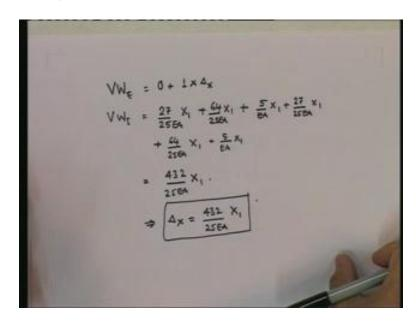
27 upon 25EA  $X_1$ , plus delta bc is going to be 64 upon 25EA  $X_1$ , plus 5 upon EA  $X_1$ , into 1 that is going to be 5 into  $X_1$ , then CD is going to be equal to 27 upon 25EA  $X_1$ , AD is going to be 16 by 6 into 4 by 5 64 upon 25  $X_1$ , plus 5 upon EA  $X_1$  into 1; this is by internal virtual work.
