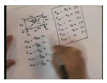
When I actually solved this, I can assume, if I take this to be the virtual force, what will be the forces in all the members? I know the forces I am going to have, so if you look at it using the method of virtual force, what is the displacement at this point? What is the displacement at this point? The displacement at this point can be given by the virtual work equation.
