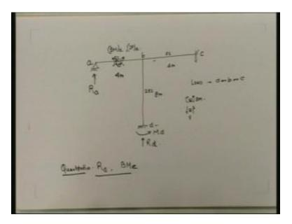
Now we are going into real examples. The load only moves in a, b and c – vertical loads only move between a, b and c. The flexural rigidity for this is EI, the flexural rigidity for this is EI and the flexural rigidity of this is 2 EI (Refer Slide Time: 03:42). We are given the fact that bending moment positive is this way and this is shear force positive – shear force and this is bending moment. This span is 4 meters (Refer Slide Time: 4:31), this is 4 meters and this is 8 meters height.
