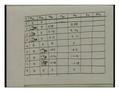
Once you know this,  $M_{dc}$  is directly this (Refer Slide Time: 36:28). Now the point that we are trying to make over here is that once you put this factor in, you can get  $R_a$  and bending moment, you can get  $M_{ba}$ . I am not going to do all of this. The overall procedure boils down to three steps. The first step is to determine where exactly your loads are. In this particular case, for example, load is going from a to c.
