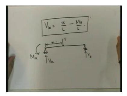
$V_b$  is going to be equal to x upon L minus  $M_a$  upon L. In this particular case, I know  $M_a$ , I know  $V_a$ , I know  $V_b$  where the load is x. Therefore, the main thing over here is that I I have found these three. The next thing that I wanted to find out was the moment and shear force at the center. Let us see how we can solve for that.
