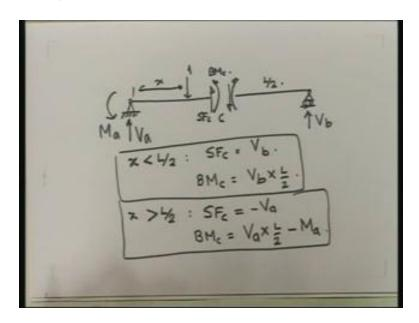
Let us look at this situation, let us assume that x... so, the shear force and bending moment are this way, this way, this is  $V_a$  (Refer Slide Time: 33:11), this is  $M_a$ , this is  $V_b$  and this is L over 2 – this length, because this is point c, this is shear force at c and this is bending moment at c. If x
