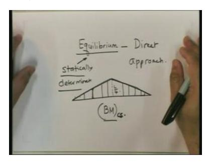
The best way and the easiest way is equilibrium – direct approach. Suppose this is my reaction (Refer Slide Time: 13:46), find it out and then plug in the values of x and find out this value. Of course, here P is equal to 1 – you have to put unit load vertical. If my bending moment in the center span was my this thing, I would put if x was less than equal to 0, this is less than L by 2 this would be the value, this would be the value if it was greater than L by 2.
