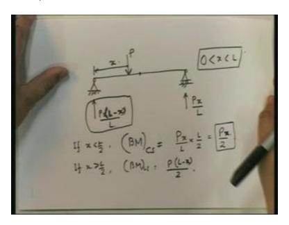
Let me put the load at a position x from the left end. Now this load is P (Refer Slide Time: 07:09) – it could be any load, put it equal to x and then find out the reaction here, the reaction here. What would be the reaction over here? The reaction over here would be Px upon L, the reaction over here would be P into (L minus x) upon L. What would be the bending moment at the center? The bending moment at the center span would be equal to Px assuming that the load
