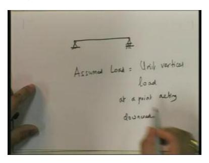
Note that whenever we are drawing influence lines, we do not have any load because what is the assumed load? The assumed load is unit vertical load at a point acting downwards. When we are looking at influence lines, we do not have a load at all because it is always unit vertical load at a point acting downwards.
