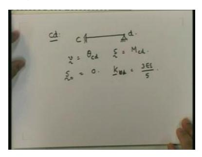
Therefore, the next consideration would be for cd; cd is continuous at c so it is fixed and at d it is hinged; this is c, d and therefore, v in this particular case is theta<sub>cd</sub>, S is equal to  $M_{cd}$ ,  $M_{cd}$  is equal to 0 (there is no load) and  $M_{cd}$  is equal to 3 EI by length which is 5. I have found out for each of the members. Now, I need to find out to how to get the member degrees of freedom related to the
