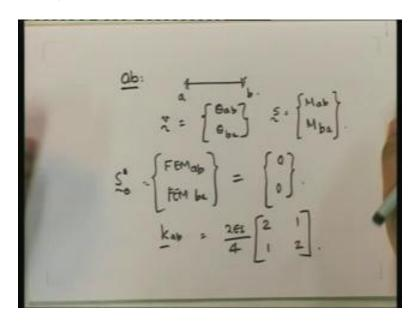
For ab, what is it? The member is fixed at a and continuous at b and therefore, v is equal to theta<sub>ab</sub>, theta<sub>ba</sub> – that is v. What is S? S is  $M_{ab}$ ,  $M_{ba}$ . (FEM)<sub>ab</sub>, (FEM)<sub>ba</sub> is equal to  $S_0$  is equal to 0, 0 and  $K_{ab}$  is equal to 2EI and this is 4 meters, this is 2 1, 1 2 – this is your member ab. Now, bc is a rigid member and therefore you do not consider bc as part of the members.
