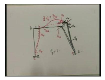
Here  $r_1$  is equal to 1. This point – where will it go? Since this is fixed, it can only move in this direction (Refer Slide Time: 09:22), so  $r_1$  is equal to 1 means b moves here. Now, this point also has to move horizontally by 1, but note that since this is an inclined member it cannot go this way so it has to move along this, so it comes over here whose horizontal component is 1 and then from geometry you will see that this is equal to 3 by 4 and this is equal to 5 by 4.
