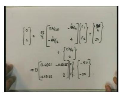
I have 0 0 equal to... now I need to do  $K_{ab}$  – it is given by this (Refer Slide Time: 30:08) and  $K_{bc}$  is given by this, so this is equal to.... I can put EI by 2 outside and inside, I will have 79 plus 48, 79 by 48 is 127 upon 128, here I have 13 by 16 and 12 by 16, so I will get minus 25 upon 16 (13 by 16 plus 12 by 16, minus 25 by 16) and here also, we will get minus 25 upon 16 and over here,
