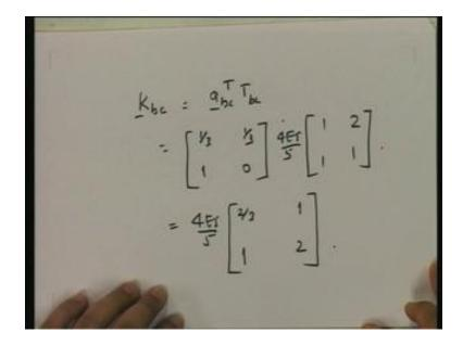
This is equal to  $a_{bc}$  transpose  $T_{bc}$ , so that is equal to (1 over 3, 1 over 3, 1, 0) multiplied by 4EI upon 5 into (1, 1, 2, 1); this is equal to 4EI upon 5, I get one-third, one-third, two-third, here I get 1, here I get 1 and here I get 2 – this is the contribution of the member bc to the structure stiffness matrix. If we put it together, let us see what we get.
