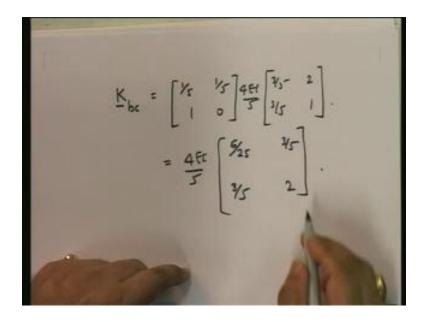
The next step is to find out  $K_{bc}$ . It is going to be equal to (1 by 5, 1 by 5, 1, 0) into 4EI upon 5 into (3 by 5, 3 by 5, 2, 1). This is going to be equal to 4EI by 5, this is going to be 3 by 25, 3 by
