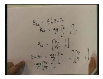
$K_{bc}$  is going to be equal to  $a_{bc}$  transpose  $K_{bc}$   $a_{bc}$ . Now,  $a_{bc}$  is equal to 4EI upon 5 into (2, 1, 1, 2)... that is  $K_{bc}$  and  $a_{bc}$  is equal to (1 by 5, 1 by 5, 1, 0). Therefore, the first thing is  $K_{bc}$  into  $a_{bc}$  and this is equal to 4EI by 5 into (2, 1, 1, 2) into (1 by 5, 1 by 5, 1, 0) and this is going to be equal to 4EI by 5; you have 2 by 5, so 3 by 5, here also you have 3 by 5, here you have 2, here you have 1.
