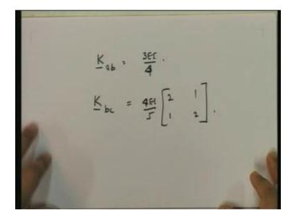
Now, we come to the Ks. They are also the same. K of ab is equal to 3EI by 4 and  $K_{bc}$  is equal to 4EI by 5 – because EI is 2 EI – into (2, 1, 1, 2) – that is the stiffness for each member.
