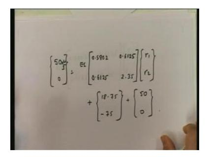
Now, I am going to put everything together and so what I have over here is r which is 50, 0 is equal to K; K is equal to EI into (0.5802, 0.6125, 0.6125, 2.35) into  $(r_1, r_2)$  plus (18.75, minus 75) plus (50, 0).
