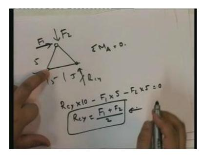
This is 5, this is 5 (Refer Slide Time: 37:09) and this is 5, this is  $F_2$  and this is  $F_1$  and I need to find out  $R_{CY}$ . Take moments about A is equal to 0. What do I get?  $R_{CY}$  into 10, this is a counterclockwise movement and both of these give rise to clockwise movement, so the clockwise movements are  $F_1$  into 5 minus  $F_2$  into 5 is equal to 0, and  $R_{CY}$  is equal to ( $F_1$  plus  $F_2$ ) by 2.
