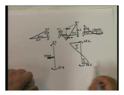
For ab, 12.3; for bc, it is 12.0, minus 62.3 and a 10 Kilonewton force acting at 10 meters, this is 30 meters, this is 30 meters, then we have cd – we have 110.7 with a udl of 1.2 Kilonewton per
