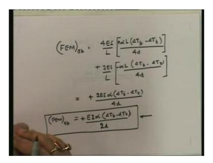
Therefore, when we substitute in here, this has to be plus and this has to be minus, therefore this becomes plus and this becomes plus. Remember that the rotation that we get is this plus this rotation has to be equal to 0. Therefore, when this is minus, this (Refer Slide Time: 18:24) plus this is going to give you 0; then this plus this is going to give you 0. Therefore, the fixed end moment here has to be positive.
