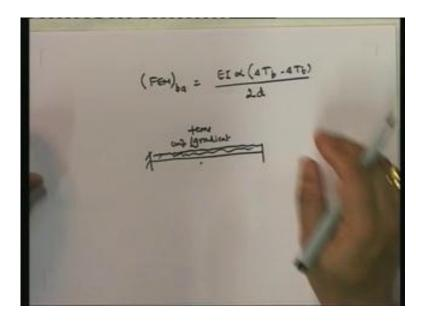
Similarly, you can actually get that the fixed end moment at ba is going to be equal to (EI alpha into (delta  $T_{bottom}$  minus delta  $T_{top}$ )) upon 2d. Therefore, if I have a uniform temperature gradient with the bottom being hotter than the top, it expands in this way so that you get it to be equal to the opposite. I would just like to make a point here: remember that theta<sub>ab</sub> is equal to minus and theta<sub>ba</sub> is equal to plus.
