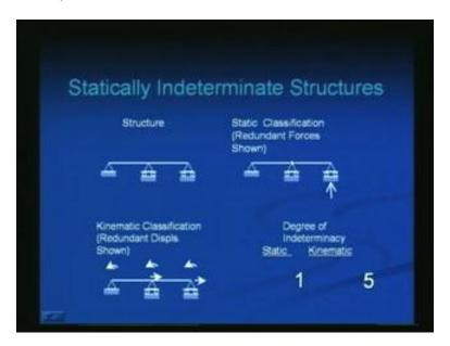
Let us look at a few other structures. This is a multispan beam. I need to find out its number of Degrees of Freedom and the Static Indeterminacy. If I remove this it becomes statically determinate so there is only one Static Indeterminacy. How many kinematic? It is 1, 2, 3 so 3 into 3 is 9. How many restraints? It is 1, 2, 3, 4 so totally 4 restraints. Then 9 minus 4 is 5. Static Indeterminacy is 1 and Kinematic Indeterminacy is 5.
