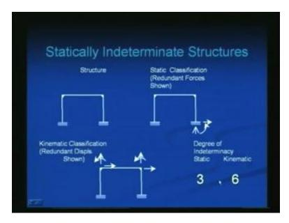
Look at the frame structure; we have already seen this. It is 3 and 6. Static Indeterminacy is 3, Kinematic Indeterminacy is 6 and that brings us to the end of this lecture. At the end of this lecture, I am going to assume from here that given any structure you should be able to find out its Static Indeterminacy and Kinematic Indeterminacy or Kinematic Indeterminacy I replace sometimes by degrees of freedom.
