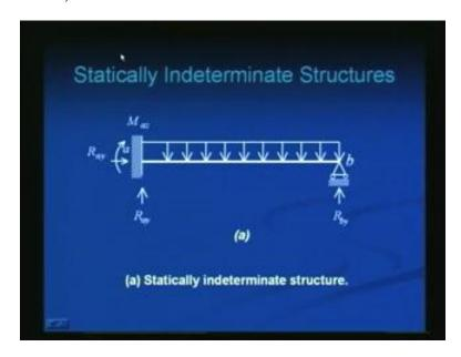
This is a propped cantilever. It is a statically indeterminate structure, because it has 4 support reactions and 3 equations of equilibrium. It is statically indeterminate structure.
