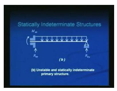
Let us look at another one. Here, what you have is this left joint which you have allowed to move horizontally. Suppose, I apply a horizontal load to this beam what is going to happen? This beam is going to move because there is no horizontal restraint. It only has two vertical restraints and a movement restraint to the left hand. This structure is unstable. Therefore understand one thing, it is very important before you start looking at Static Indeterminacy, you need to know whether it
