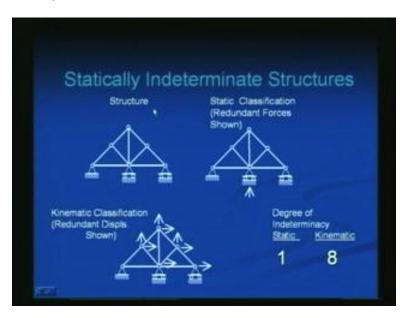
For a truss, remember that each one is triangulated so it is internally determinate and if I remove one of these it becomes 3 and becomes externally determinate also. This is the only redundant
