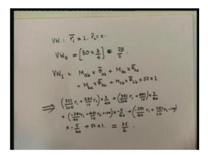
I am going to put the first virtual work equation as  $r_1$  is equal to 1; since it is in an arbitrary displacement pattern, the first displacement pattern is going to be this pattern. My external work will be the load into 1. What is the external load? There is only one external load, which is 50 tons because that is applied at the joint. How much displacement does that undergo?
