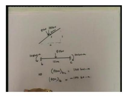
Note that there is a slight difference here: the member is inclined and the loading is this way, so I can actually write this load of 100 Kilonewton. This is a 3, 4, 5 triangle and therefore, if I write down the vertical component and then the horizontal component, the vertical component of this is going to be 80 Kilonewton and the horizontal component is going to be 60 Kilonewton.
