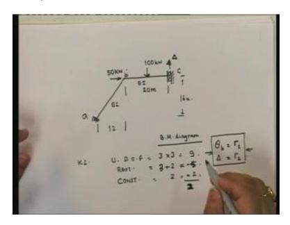
First, the degrees of freedom. Determine the kinematic indeterminacy. How do we go about it? 1, 2,3, so how many joints? The unrestrained degrees of freedom are equal to 3 into 3, 9. How many restraints? This is the fixed (Refer Slide Time: 47:19), so in a fixed you have two; and this
