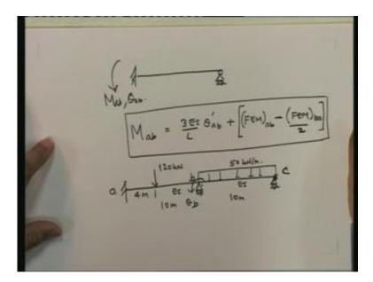
Ultimately, if you look at the equation for this, it turns out to be  $M_{ab}$  is equal to 3EI upon L into theta (this is where you take it from the chord plus and here, I am going to write down the expression for the fixed fixed case – these are the fixed end moments from the fixed fixed case; and this is algebraic – if the sign of ba is different from ab, it becomes positive. This becomes my new equation; I am going to use this to solve a problem that we had solved earlier.
