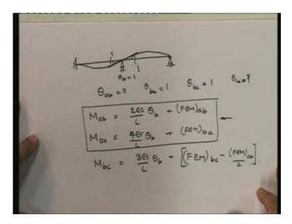
Note that that is the only degree of freedom so this is going to become 1. I am going to have a displacement pattern that looks like this and note that over here, it does not have to go to 0 because this is a hinge and it can take any value.
