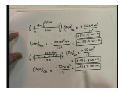
These were the fixed fixed, so ab is equal to plus 172.8, (FEM)<sub>ba</sub> is equal to minus 115.2 and (FEM)<sub>bc</sub> is equal to 416 and minus 416. Having done that, I can plug in those values directly. Therefore, what do I get?
