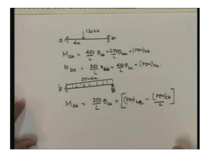
What we are going to do is, we going to be considering ab as a fixed fixed. As far as ab is considered, we are going to say  $M_{ab}$  is equal to 4EI upon L theta<sub>ab</sub> plus 2EI by L into theta<sub>ba</sub> (note that since there are no displacements, I am not even writing down the delta because the
