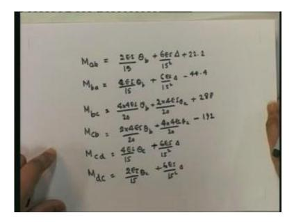
$M_{ab}$  as 6 plus 6, then I have  $M_{cd}$  has 6 plus 6, so this is going to become equal to 24EI by 225 delta and then, I have 22 minus 44, that is minus 22, minus 22 minus 300, so this is going to be equal to minus 322.2 is equal to 0. Now, I have three equations. I will just put it down finally in an equation format.
