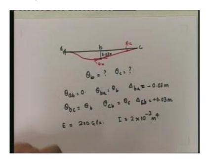
What you have is this, the support has settled and the support settlement is 0.03 meters. So, what will the deflected pattern look like? This is theta<sub>c</sub> (Refer Slide Time: 02:15) and this is theta<sub>b</sub> – the two unknown rotations, the two displacements corresponding to the degrees of freedom; so, theta<sub>b</sub> is unknown, theta<sub>c</sub> is unknown.
