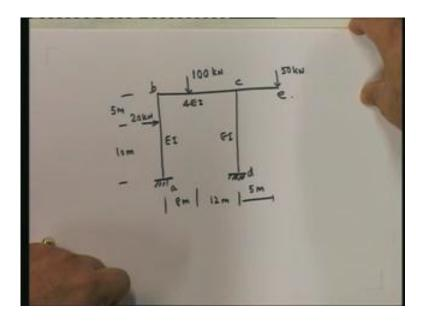
This is a frame that we have and if you look at this particular frame, it has fixed supports at a and d and it is a single-storey, single bay frame with an overhang. At the end of the overhang, you have a load, you have one load in member bc; member ab has a load, bc has a load, ca has a load and cd has a load. In this particular case, you will see that I am going to eliminate ce because I am not quite interested. If you look at ce, can I draw the bending moment diagram for ce? Sure, I can.
