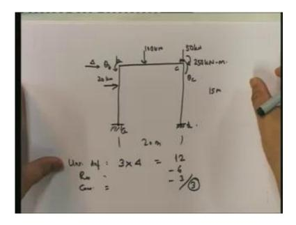
I can solve this problem. 15 meters, 20 meters, load here (Refer Slide Time: 21:12), load here and this load, I can transfer here as 50 Kilonewton, but just transferring the load is not good enough. What happens? Equivalent load system, I also have to transfer a moment and the moment is equal to 250 Kilonewton meter (Refer Slide Time: 21:29). Now, I am solving abcd. This is the problem that we have to solve using the displacement method.
