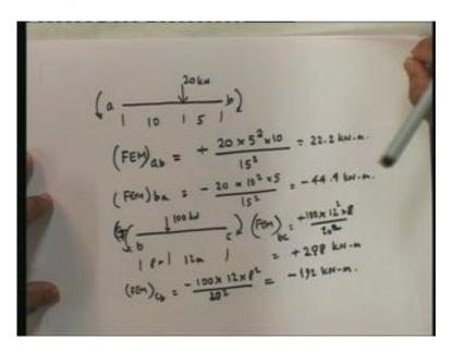
Member ab has a load. What is the load? This is a, b, 10 meters, 5 meters; at this point, we have a 20 Kilonewton force. What is this going to give me? The fixed end moment at ab is going to be equal to b and note that this is going to be this way (Refer Slide Time: 32:51) and this is going to be this way; this is positive, so this is going to be plus ((20 into 5 squared into 10) by 15 squared); this is going to be equal to 22.2 Kilonewton meter.
