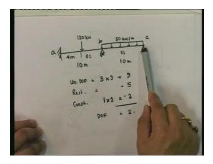
Given this loading on this multi-span beam, we use the displacement method to generate the shear force and bending moment diagram. To take it forward, let us look at another aspect of this particular problem and that is, what do we do when we have support settlement? Remember that I talked about support settlement when we looking at the force method. Let me take this particular problem itself.
