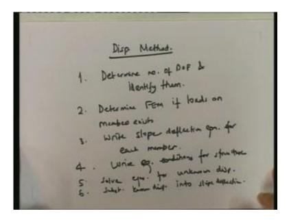
One: determine the number of degrees of freedom and identify them; two: determine the fixed end moment if loads on members exist; three: write the slope deflection equations for each member; four: write the equilibrium conditions for the structure; five: solve the equations for unknown displacements; and six: substitute the known displacements into the slope deflection equations so that you can get your member end moments and once you get your member end moments, you should be able to solve it.
