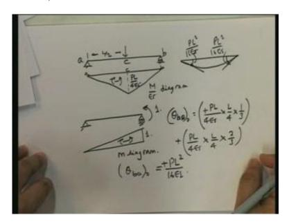
Under the same loading, this is acting at L by 2, same M by EI diagram, I am just drawing it all over again. This is my M by EI diagram and now I want to find out.... This is a, this is b, this is c, a, c, b (Refer Slide Time: 22:14). Now, I want to find out theta<sub>ba</sub>. What do I do? I
