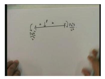
When you substitute, you will get.... This is P, put a and b, you will get that this is equal to P into a b squared by L squared and this turns out to be P a squared b upon L squared; now, substitute. If you want to check, put a and b as L by 2, L by 2 and you will get PL upon 8, PL upon 8, which is what you got earlier. I am going to stop over here.
