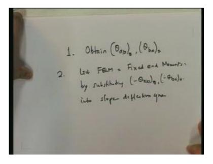
First, take the simply supported and obtain theta<sub>ab</sub> and theta<sub>ba</sub> due to the loading. Two, get the fixed end moments (this is fixed end moments; this is my notation) by substituting minus (theta<sub>ab</sub>)<sub>0</sub> and minus (theta<sub>ba</sub>)<sub>0</sub> into the slope deflection equations. Let me again take this.
