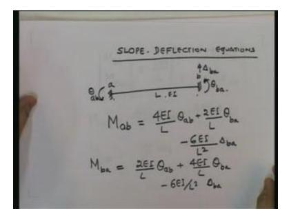
4 EI upon L theta<sub>ab</sub> plus 2 EI by L theta<sub>ba</sub>. Forget this term for now. These two terms, I have just developed. These terms have not been developed because I did not consider this delta. I only considered theta<sub>ab</sub> and theta<sub>ba</sub> to occur due to  $M_1$  and  $M_2$ . Now, how do I include this? Simple. Bear with me and I will take you through this. These two terms (Refer Slide Time: 27:30), this
