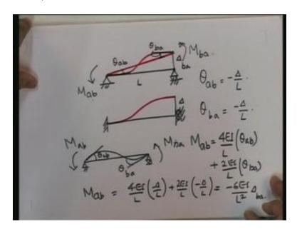
Take this situation; this is a pin here and a pin here. Suppose I were to remove this and let this go up by delta. Note that this delta is small compared to the L and so it is essentially a small displacement. How would this displace? Note that this is free to rotate. So, if you look at the displacement pattern for a simply supported beam it would just be this, it will be a straight line where this angle would be delta upon L. Now, let us look at the system that we were looking at, the original.
