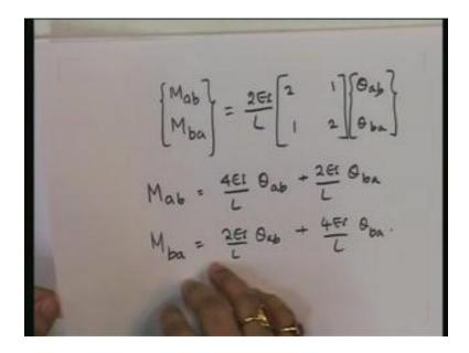
If I rewrite, plug this into here, what I get is  $M_{ab}$ ,  $M_{ba}$  is equal to 2 EI upon L 2, 1, 1, 2 into theta<sub>ab</sub>, theta<sub>ba</sub>. If I write this in a proper format, it will become  $M_{ab}$  is equal to 4 EI upon L theta<sub>ab</sub> plus 2 EI upon L theta<sub>ba</sub>; and  $M_{ba}$  is equal to 2 EI upon L theta<sub>ab</sub> plus 4 EI upon L theta<sub>ba</sub>. Simple. If you look back at the slope deflection equation, what did I write down?
