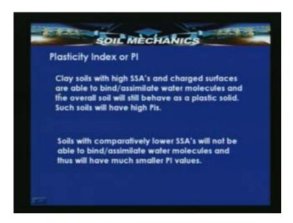
Clay soils with high specific surface area and charged surfaces are able to bind and assimilate water molecules and the overall soil will still behave as a plastic solid. Such
