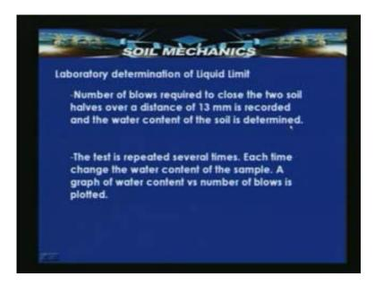
Number of blows required to close the two soil halves over a distance of 13mm is recorded and the water content of the soil is determined. So the test is repeated several times that is what being discussed. The test is required to be repeated at different water contents and the number of blows which are required to close 13mm groove is required to be measured. Each time the change in the water content of the sample is noted the graph of the water content versus the number of blows is plotted.
