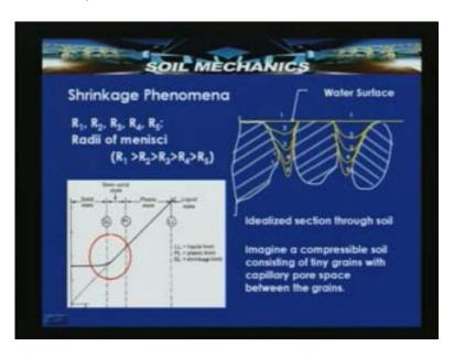
Let us consider the grains which are shown here, an idealized section through the soil, assume that these are the grains and these are the different water surfaces which are shown with different stages 1, 2, 3, 4, 5. When the soil changes from semisolid to solid state in this curvilinear zone the water gradually gets replaced with air. Let us assume that a compressible soil consisting of tiny grains that means grains as small as possible with capillary pore space between the grains.
