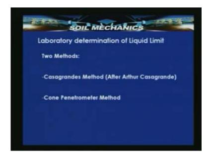
Liquid limit is basically determined in the laboratory by using two widely accepted methods. One is Casagrandes cup method, it is also called Casagrandes method. This is
