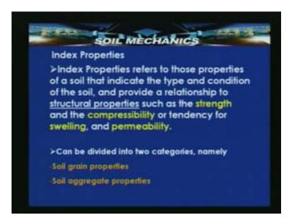
Basically these soil index properties can be divided into two categories, they are: soil grain properties and soil aggregate properties. The development of the ability to think of soils in terms of numerical values of their index properties should be one of the foremost aims of every engineer who deals with Soil Mechanics.
