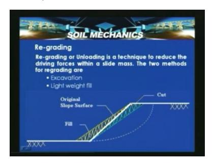
Now here which is shown, another option is that this portion of the slope was removed and then provided here which actually makes the slope flattened slightly. Lowering of ground water to reduce pore pressures in the slope. so that is nothing but the portion for drainage of a slope, here interceptor ditches for diverting the surface slopes that actually helps here and these are the collector drains with perforated pipe in gravel filter envelope.
