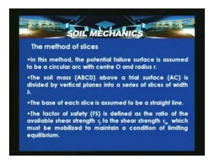
Now let us consider a slope cross section having certain slope inclination and ABCD is the portion of the soil which is subjected to say movement. So here ABCD is the slope portion, previously in the circular arc method what we did is that we try to find the weight area of the entire portion and then multiplied by its unit weight.
