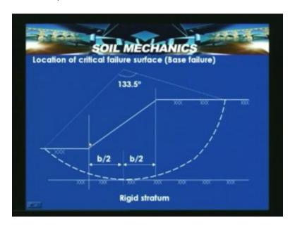
Now having looked into it, particularly this stability analysis which is required to be carried out for short term and long term conditions. So short term stability basically this is carried out for a low permeability soils where the drainage is not permitted and long term conditions where the fully drain stage can occur, in that case c dash and phi dash parameters are required to be used.
