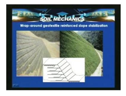
So in this case a wrap around geo textile info slope is shown and after about certain time you can see how that green esthetic view of the look. So this type of techniques can mingle well with environment. So this is another type of slope stabilization technique which can be used for retaining this and which also is gaining momentum in its application.
