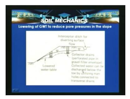
So the lowering of the ground water table to reduce the pore water pressure in this slope is another option which is actually done through surface interceptor ditches or collector drains within the slopes. So drainage reduces the destabilizing hydrostatic and seepage forces on a slope as well as the risk of erosion and piping. So it can be surface drainage and sub-surface drainage.
