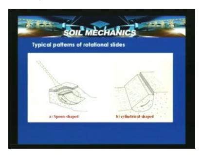
There is a settlement or a depression from this level and then down the movement of the slope takes place. In the method of slices the potential failure surfaces assumed to be circular arc with a centre of rotation O and its radius r and how to locate this critical failure surface that we look into it later.
