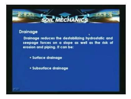
The drainage phenomenon which reduce the destabilizing hydrostatic and seepage forces on a slope as well as the risk of erosion and piping. Plan for building design to aid slope stability, suppose if the building design is made like this if at the crest of the slope a building is constructed and similarly at another building is constructed at the toe of the slope, the shallow foundations or basement for the building or below the toe and deep foundations or basement for the building on the slope.
