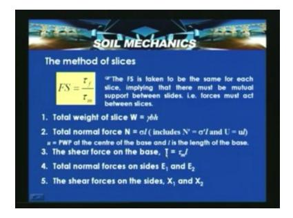
Once again let us look into the free body diagram  $E_1$  and  $E_2$  which are shown here and  $x_1$  and  $x_2$  which are shown here and this alpha is that inclination which makes with the line passing through the weight of the slice. So the weight of the slice is assumed to be center line and this is located at a distance r sin alpha from point of rotation O horizontally, so this is that I length along the base of the slice.
