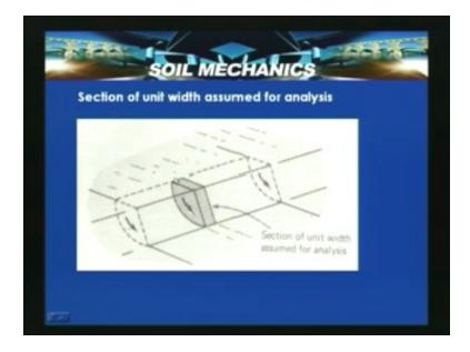
So the length of this section is assumed as for example if the weight is calculated in meters then we calculate the weight of this section per meter width of this particular reaction. So if this is the slope, this is that section of unit width assumed for analysis and that is considered because this type of structures or this thing illustrates a plane strain condition.
