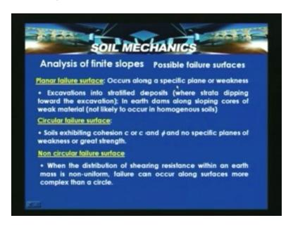
In earth dams along sloping cores of weak material not likely this particular, this planer failure surface may not likely to occur in homogeneous soils. So in stratified deposits or examples like earth dams where there is a sloping core of weak material, core material which generally comprised of low strength material but which is having impervious characteristics.
