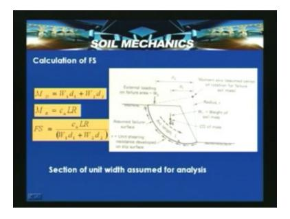
Now let us look the driving moment which can be given by  $w_1$   $d_1$  plus  $w_2$  into  $d_2$  that is moment about this point. Resting moment is now only  $c_u$  into L into R. So factor of safety is nothing but a ratio of resting moment to driving moment which is  $c_u$  LR divided by  $w_1$   $d_1$  plus  $w_2$  into  $d_2$ . So even in the loads which are considered the per meter or per unit width of the analysis is considered and which yields factor of safety.
