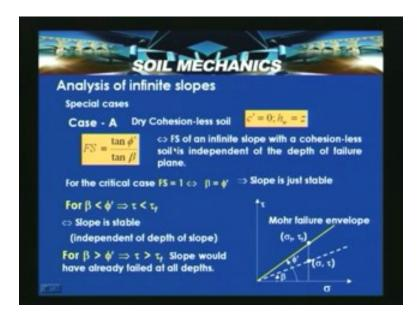
So for critical case the factor of safety is equal to one so beta is equal to phi dash, the slope is just stable; for beta less than phi dash that means the driving shear stress are less than the available shear strength. Let us look this in the tow sigma plot, let us consider a tow sigma plot which is shown here and slope inclination is indicated with broken line here and Mohr failure envelope is indicated with yellow line which is shown here.
