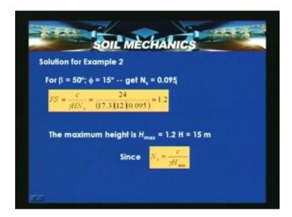
Factor of safety is equal to c divided by gamma H  $N_s$ ,  $N_s$  is the stability number which is obtained as 0.095 based on the given data. So 24 divided by 17.3 into 12 into 0.095 which yields factor of safety 1.2 that's what we are required to determine in this problem, what is the factor of safety in regard to cohesion only. So the maximum height  $H_{max}$
