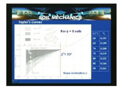
So here different types of circles are passed like slope circle, toe circle and base circle, the zones are indicated here. This is valid for beta less than 53 degrees and the depth factor cannot be ignored but beyond that this indicates that the depth factor will not come to picture. So this particular curve is for  $phi_u$  is equal to zero soils that means these are for the un drained condition that is  $c_u$  that is purely cohesive soils or saturated cohesive soils.
