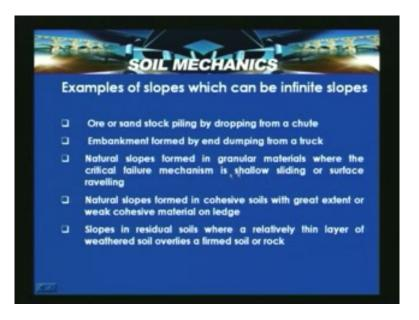
So in this translational slide, failure of a slope along the weak zone of soil so in this case there is a thin layer of weak soil if it exists and that can induce a translational slide. Sliding mass travels long distance before coming to rest and common in coarse grained soils.
