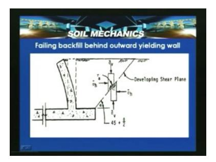
So we also discussed about a Mohr strength diagrams, here the development of the Mohr strength diagram during the progressive outward wall direction is shown here.
