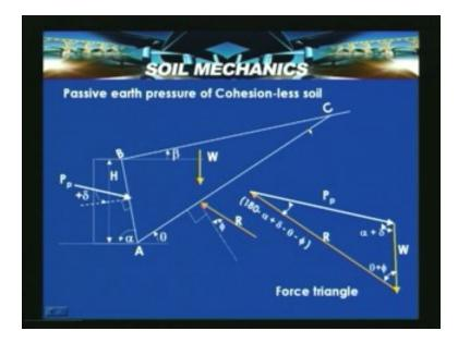
Now beta is the backfill surface inclination and theta is AC is the inclination of the potential surface where here in this case passive case where the one which gives the minimum value that need to be considered.
