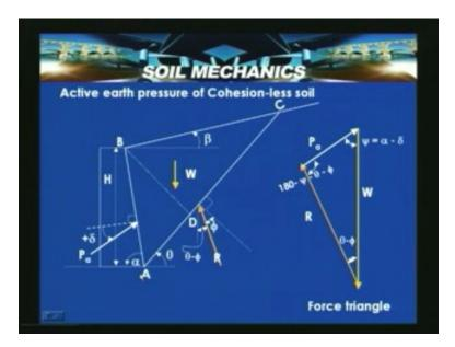
So this position of the active thrust which is assumed like this, if this is the cg and if this located at this point, a line passing through this say failure surface which is inclined at theta which gives the location of the active thrust that is at this point. So the same forces like W and this R and P<sub>a</sub> which are acting on this triangular wedge ABC for the active case when the wall moves away from the backfill can be represented in the force triangle like this.
