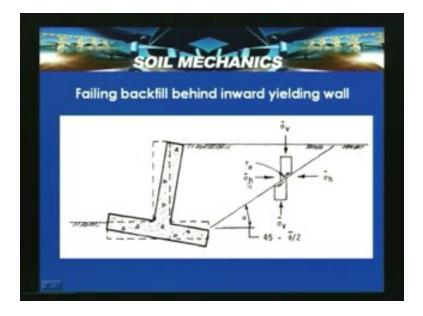
So this retaining wall is yielding towards the backfill so induces a compression in this case where along this shear plane it actually induces tow alpha that is the shear stress which gets mobilized and the wedge of the failure. So sigma<sub>v</sub> and with the vertical stress and sigma<sub>h</sub> is the horizontal stress. So in this case the sigma<sub>h</sub> becomes the major principle stress, sigma<sub>v</sub> becomes the minor principle stress.
