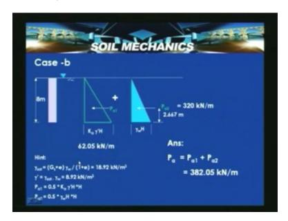
So as it actually rises from the bottom so actually induces instability to the wall, if it is not designed if it is not drained properly. So now the net pressure is now 382.05 that is about 3 to 4 times there is a increase in the lateral active thrust on the wall with an raising water table. So the effect of the ground water surface on the active thrust can be noted here. So a case where suppose you have got a soil and then which is actually prone for say capillarity saturation.
