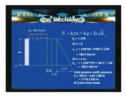
So with that what will happen is that  $k_p$  for a given friction angle, we can obtain at z is equal to zero, sigma $_p$  is equal to 1.698 into 50 plus 2 in to 40 into root over 1.698 which actually yields 188.9 kilo newton meter per square that is at z is equal to zero because this is a passive case wall moves towards the backfill so 1.698 into 50.
