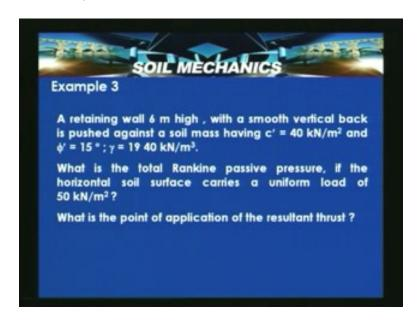
So what we can do is that surcharge is 50 kilonewton meter per square, wall is height of 6 meters Rankine case but wall moves towards the backfill. So it indicates the passive case now, sigma<sub>p</sub> is equal to  $k_p$  gamma z plus  $k_p$  q plus 2c root  $k_p$ .
