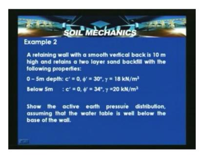
So basically we need to show the active earth pressure distribution assuming that the water table is well below the base of the wall and here we have 2 types of soils and up to 5 meters and below 5 meters there is another type of soil. So this particular case is illustrated here so c dash is equal to zero, phi dash is equal to 30 dash,  $k_{a1}$  is obtained 0.33 from 30 degrees friction angle 1 minus sin 30 by 1 plus sin 30. So 1 minus sin 34 by 1 plus sin 34 that is for  $k_{a2}$  it is 0.283.
