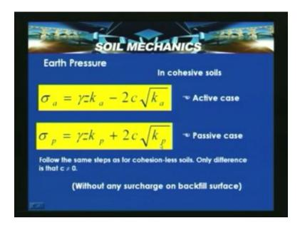
So with this now the generalized equations without any surcharge on the backfill surface if you consider then these are the generalized equations for computing the earth pressure. Then sigma<sub>a</sub> is equal to gamma z ka minus 2c root  $k_a$  this is the active state and sigma<sub>p</sub> is equal to gamma z  $k_p$  plus 2c root  $k_p$  that is for the passive state. So follow the same steps as cohesion less soils, only difference is that c dash is not equal to zero.
