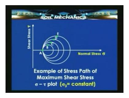
Here is another example of stress paths. We do a lot of tests continuously one after the other on a same specimen but with constant sigma<sub>3</sub> and only sigma<sub>1</sub> goes on changing and again let us take the maximum shear stress point those will be at constant sigma<sub>3</sub> A B C D E.
