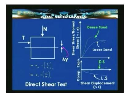
If it is a loose sand it will under compression continuously. There will be a peak shear stress and an ultimate shear stress as the displacement increases. The same thing can be observed in a triaxial test also, for dense sand there is a peak, for loose sand there is no marked peak. Loose sand undergoes compaction or compression, dense sand undergoes a little bit of compression initially but then undergoes expansion subsequently, it becomes loosened.
