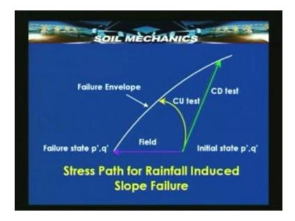
Here we have the stress path which actually exists during rainfall. This arrow going from right to left shows how the initial values of p dash and q dash gradually change to the final failure state p dash q dash with total stress remaining same. So this is the true stress path in the field. The soil
