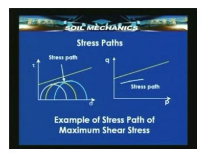
Here is an example of a stress path which is showing how the maximum shear stress is varying as loading changes in typical triaxial test. Here is the sigma tow plot and here is the corresponding p q plot. From the sigma plot we know very well that if 3 tests are conducted 3 triaxial test, 3 successive Mohr's circles can be obtained and if I take the stress state corresponding to the maximum shear stress that will obviously be the point at the top of the semicircle here.
