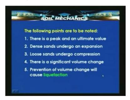
One there is a peak and an ultimate which we saw in the previous diagram. Dense sands undergo an expansion mostly although they undergo a little bit of compression initially, loose sands undergo compression. There is a significant volume change the amount of compression or the amount of expansion is quiet significant under shear.
