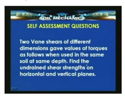
Now suppose if you have 2 different vanes and you test the same soil for strength with these 2 different vanes, how do we get the shear strength of the soil in the horizontal and the vertical direction planes? This can be done by going back to fundamental equations of torque generated in a vane shear test.
