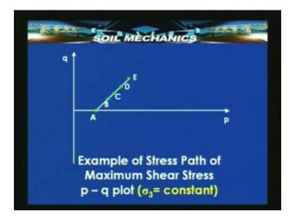
If you now plot them on the p q graph, you get a straight line at 45 degrees and this is nothing but a maximum shear stress path corresponding to sigma<sub>3</sub> constant state.
