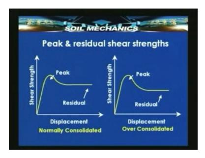
If you take a normally consolidated soil, you will have a shear strength verses displacement curve which will be something this which shows a peak. Then it comes down and shows a residual value, with large displacements the value goes beyond and then comes down and remains almost constant. So is the case with over consolidated clays also. There is a peak and then a residual value but what is obvious from these two figures is that when the soil is over
