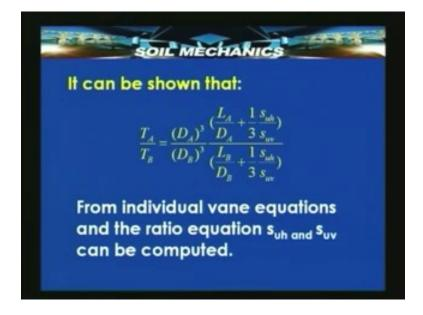
By using the individual equations for torque for each vane and the ratio of the torques and by knowing the geometry of the vanes, one can easily determine  $S_{uh}$  and  $S_{uv}$  which are the required shear strengths in the horizontal and the vertical directions.
