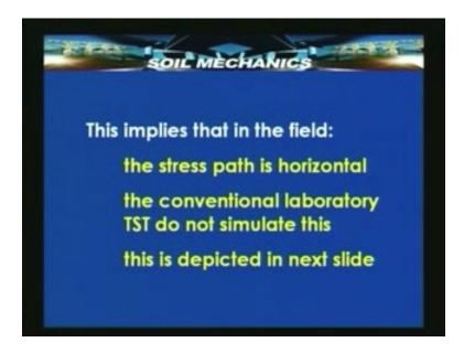
The conventional laboratory test unfortunately does not help you to simulate this horizontal stress path and therefore we will have to device a special testing technique, cyclic triaxial test could probably be an alternative. In the next slide we will see how the stress really varies, what kind of stress path we get in our conventional test and what should be the real stress path that should be simulated.
