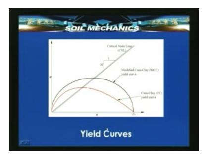
Here are the yield curves which will result if we use the cam clay model. Here is the yield surface on the p q plot for cam clay, this is for the modified cam clay and this is the line which tells us which are those critical stress state at which a soil will either according to cam clay model or according to the modified clay model corresponds to a situation where there is yield or there is a large deformation.
