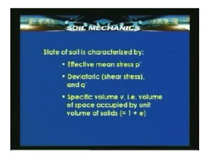
As in the Drucker Prager theory we had 2 parameters, here we have 3 parameters. The Mohr coulomb theory has again only 2 parameters c and phi. The cam clay model on other hand uses p dash and of course q dash but it also uses the specific volume v.
