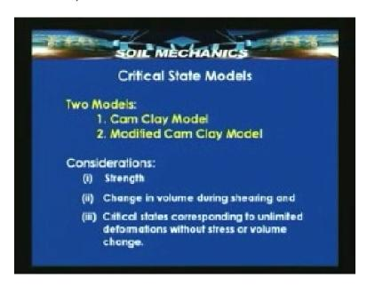
One model is of special interest and it is worth making a mention about it although not much in detail. This is known as the critical state model. There are two different models proposed under this, one is known the cam clay model another is known as modified cam clay model. These were proposed by Andrew Schofield in Cambridge.
