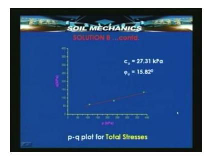
Here the p q plots are shown and the  $c_u$  and  $phi_u$  values corresponding to total stress p q plots are also displayed.
