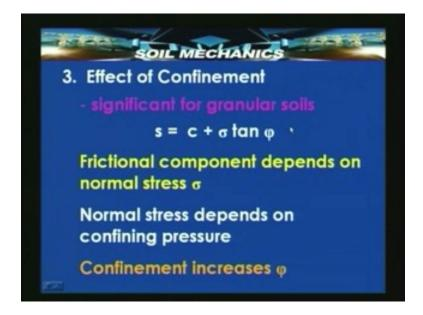
Now confinement is also again significant for granular soils, the frictional component depends upon the normal stress sigma and the normal stress sigma depends upon the confining pressure where sigma is the normal pressure on any potential plane of sliding. Therefore confinement increases phi.
