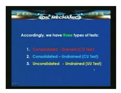
We have three combinations, well known combinations of test. The consolidated drained, consolidated undrained, unconsolidated undrained. The first is commonly called the CD test, the second one the CU test, the third the UU test or sometimes these are also known as the S slow test and the Q the quick time test.
