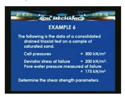
There was an example in which we had the cell pressure, the deviatoric stress at failure and the pore water pressure known and the shear strength parameters were to be determined.
