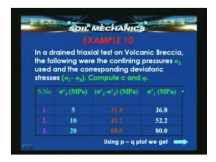
This is the summary of the results. This is again another example which we saw last time where sigma<sub>3</sub> dash and the deviatoric stress effective were both known from which we calculated the sigma<sub>1</sub> dash and computed c and phi by an effective stress p q plot.
