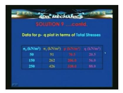
These are the data for the corresponding p q plot and the p q plot also gives you for total stress a value of  $c_U$  and a value of  $phi_U$  and for effective stresses also a value of c dash and phi dash.
