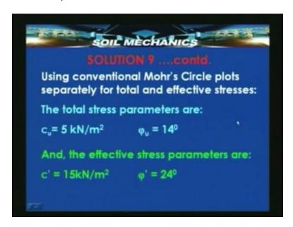
We get the values of  $c_u$  and phi u or c dash and phi dash depending upon whether we plot total stress diagram or effective stress diagram.
