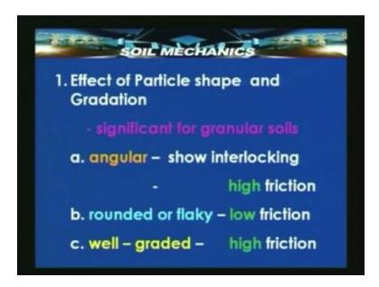
Effects of particle shape and gradation- significant only for granular soils. If the particles are angular if they have sharp edges then they exhibit lot of interlocking. Therefore the angle of friction would be high. If on the other hand they are rounded as in the case river bound soils or flaky as in the case of clayey soils, the friction is likely to be very low. And coming to gradation a soil which is well graded obviously will have the highest possible frictional resistance.
