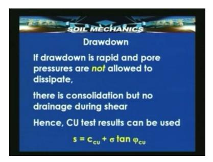
There is consolidation because sometime has passed since the dam has been constructed but there is no drainage during shear. Hence the consolidated undrained test would fit the requirement and shear strength will be  $c_{cu}$  plus sigma tan  $phi_{cu}$ .
