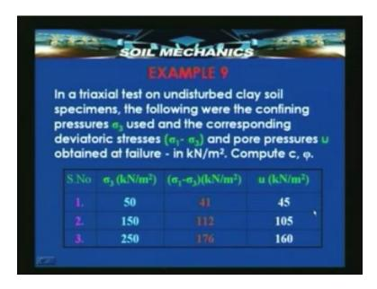
Example 9 again involved knowing sigma<sub>3</sub>, sigma<sub>1</sub>-sigma<sub>3</sub>and the pore pressure and the computation of the shear strength.
