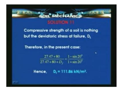
And so from the Mohr diagram and by using this relationship which can be obtained from geometry, we can get the deviatoric stress  $D_f$  which is nothing but the compressive strength. This is similar to a problem which we saw in the lecture number 3 and therefore I would recommend that you take a look at the formula and its application as it has already been discussed in lecture number 3.
