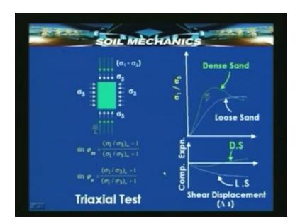
Now if you take the triaxial test again dense sand and loose sand will behave in a similar manner. If we plot sigma<sub>1</sub> upon sigma<sub>3</sub> and the shear displacement or the axial displacement in this case, we will get a diagram very similar to what we got for the direct shear test and this again shows
