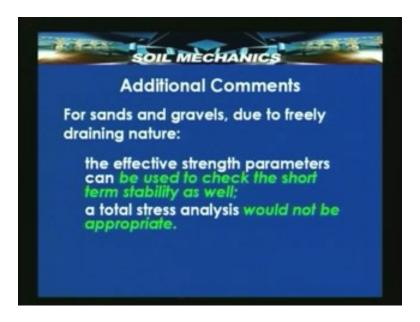
For clayey soils a total stress analysis is the only correct way to access the stability. Now there are a number of factors other than this drainage which affect the shear strength of a soil. Primarily we can identify 6 such factors.
