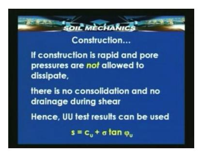
Hence it is a consolidated drained situation and CD test results can be used that is shear strength of the soil will be c dash plus sigma dash tan phi dash along any particular plane. If now consider the case of construction being done rapidly. Then pore pressures are generated and are not allowed to dissipate. There is therefore no consolidation and therefore no shear drainage during shear.
