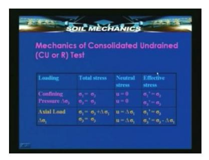
And now the effective pressure is less than the effective pressure that existed before the application of this undrained load because during undrained load pore pressures are developed and therefore whatever preexisting effective stress was there at the end of the first stage loading, gets reduced due to this additional pore pressure. So sigma<sub>1</sub> dash become sigma<sub>3</sub>, sigma<sub>3</sub> dash becomes sigma<sub>3</sub> minus delta sigma<sub>1</sub>.
