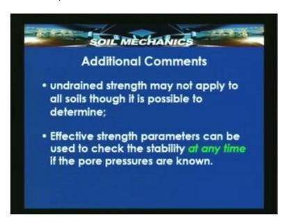
On the other hand if it is a pervious sand or gravel then effective strength parameters can still be used because pore pressures would not be allowed to generate. A total stresses analysis would not be therefore recommended for such soils.
