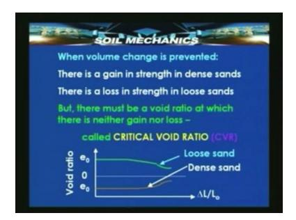
Whereas on the front of loose sands, if we do not permit volume change we are preventing the sand from becoming denser and gaining more strength. Therefore it actually loses strength but this shows that there must be a void ratio at which sand neither is dense nor is loose and
