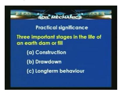
The practical significance of drainage can be very nicely understood from the example of the lifetime performance of an earth dam or a fill. So let us take the example of an earth dam. What are the major stages in its lifetime? First is the construction, as you know an earth dam is
