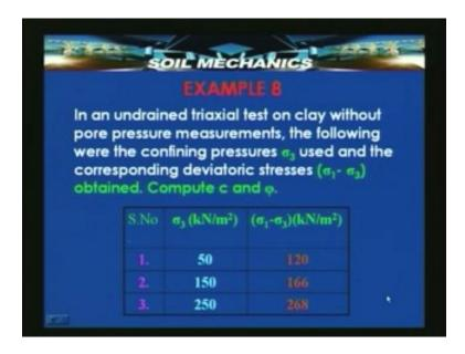
And another example 8 in which we had sigma<sub>3</sub> and the deviatoric stress sigma<sub>1</sub>-sigma<sub>3</sub>. We computed c and phi either using the Mohr's circle plot or both by using the Mohr's circle plot and by using the p q plot.
