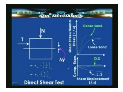
The volume slightly decreases, there is a slight compression initially and then the soil starts expanding if the soil is dense sand. On the other hand it continues to show a compression if it is loose sand and which means that we will have peak value of tan phi equal to tow upon sigma peak or a tow upon sigma ultimate corresponding to the portion beyond the peak. And in the case of loose sand only the second aspect will apply.
