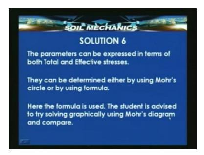
We could either determine the total stresses or the effective stresses and using either the Mohr circle or a formula we could get the cohesions and friction.
