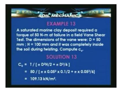
We saw a simple example where the undrained cohesion of the soil was computed from the torque and the geometrical dimensions which were available to us in this problem.
