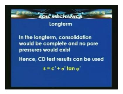
In this test as we had pointed out or seen a little earlier, the pore pressures are known. They are simply equal to the additional axial load applied during the undrained stage, the second stage of loading. Since the pore pressures are known although we get the total stresses and shear strength parameters corresponding to the total stresses, we can always easily the effective stresses and the effective stress parameters and use them. And in fact often this test is preferred to the simple
