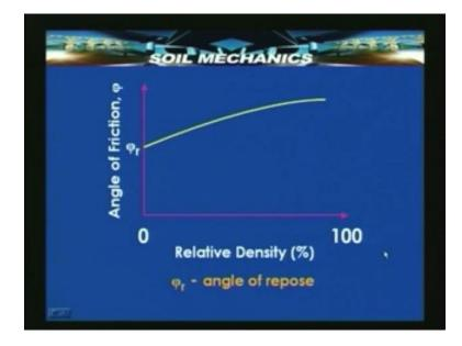
There is approximate relationship between the angle of friction and the relative density, as the relative density percentage increases from 0 to 100, the angle of friction also increases as shown in this figure.
