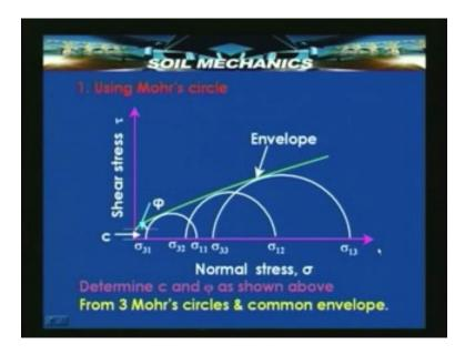
Here is the Mohr's circle plot and from the Mohr's circle plot and using the analytical relationship and also by using the p q plot, we got the values of cohesion and friction.
