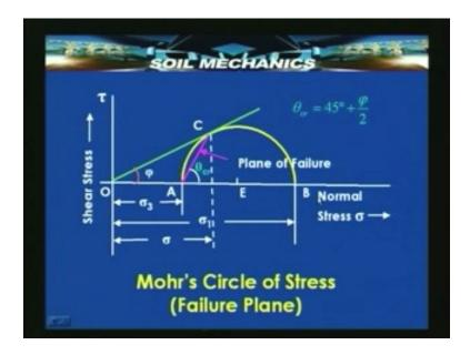
Here is the Mohr circle, by drawing the Mohr circle we can get the cohesion and friction corresponding to this envelop and if it is drained test, c will be zero.
