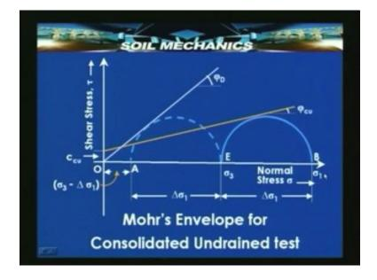
The corresponding Mohr's diagram if we take a look, the continuous line thick circle represents the total stress circle that is the total stress sigma<sub>3</sub> applied and the corresponding total stress sigma<sub>1</sub>. If we know the pore pressure which incidentally is equal to delta sigma<sub>1</sub> that is the additional axial load applied that's which the pore pressure is known in this particular test.
