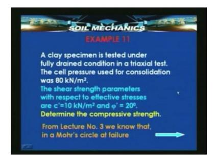
Now we go on to another example in which a clay specimen is tested under fully drained condition in a triaxial test. The cell pressure used was 80 kilo newton per meters, the shear strength parameters were known c dash and phi dash. What is the compressive strength? The compressive strength can be calculated as equal to the distance AB the deviatoric stress.
