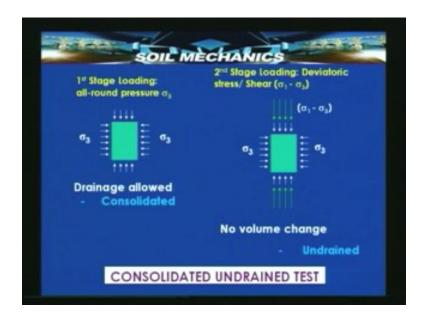
Therefore we get total stress parameter in this because unless the drainage is permitted the stresses don't become effective. Like last time if we take a look at this diagram, we find that in the first stage drainage is allowed, consolidation is permitted whereas in the second stage it is undrained during the application of the deviatoric test.
