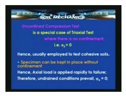
This test as you know is a special case of a triaxial test the difference between the triaxial test conventional triaxial test as it is called and this test is that the confining stress sigma<sub>3</sub> is zero. Hence it's necessary that the sample should be able to stand in the apparatus without confinement. Such a soil which will yield a sample in soil which can stand in the apparatus
