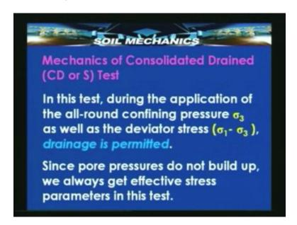
The mechanics of the consolidated drained test is very simple. In the first stage of loading that is the application of confinement, drainage is permitted and then the second stage when shear stress is applied volume change is permitted that means in effect drainage is allowed that's why this permits consolidation to take place during the first stage of loading and drainage to take place during the second stage of loading and that's why it is called consolidated drained test.
