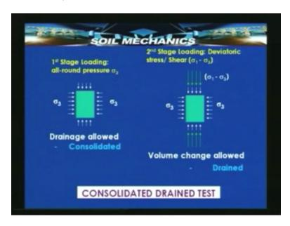
This implies that the loading is slow enough to allow water to expel and not build any pore pressure. With a help of the diagrams which we had seen a little while earlier, we can say that in the first stage drainage is allowed and consolidation is permitted and in the second stage volume is change is allowed and drainage is permitted.
