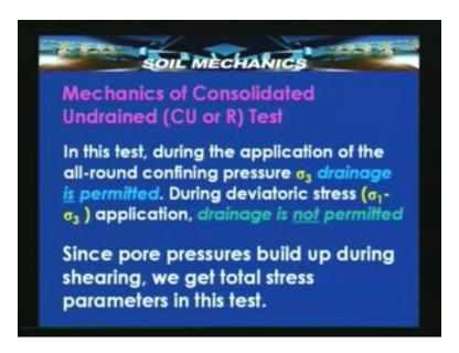
Now let us take the next test that is the consolidated undrained or R test, it is also called the R test. The difference between this and the previous test is here consolidation is permitted in the first stage of loading but in the second stage of loading drainage is not permitted, volume change is not allowed.
