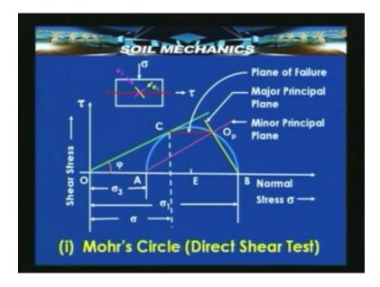
For example if you see this small rectangle this is the sample, there is horizontal plane of failure. In normal stress sigma is applied and a corresponding shear stress tow is applied until this fails.
