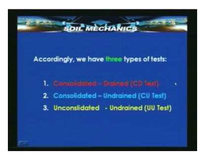
Accordingly we have 3 types of tests, first one is consolidated drained test, second one is consolidated undrained test. The last one is unconsolidated undrained test. We do not use the unconsolidated drained test that combination because it is not a realistic one, it doesn't normally happen in the field. The names which are normally used for these tests are CD, CU and UU. Now let's see the mechanics of these tests.
