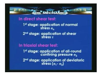
And as you know sigma<sub>3</sub> will get applied equally at the top and bottom as well because the specimen is kept in a Perspex container carrying water. And then subsequently increasing sigma<sub>3</sub> to its final value sigma<sub>1</sub> that corresponds to the application of the second stage of loading that is the deviatoric stress sigma<sub>1</sub>- sigma<sub>3</sub> half of which corresponds to the maximum shear stress.
