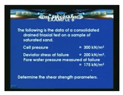
Here is an example we have the cell pressure, the deviatoric stress and we also have the pore water pressure that's the difference between a triaxial stress and a direct shear stress. The pore
