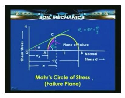
Here is a typical Mohr's circle for a triaxial test here is sigma<sub>1</sub> and sigma<sub>3</sub> we can plot the Mohr's circle, plot the envelop and get the angle of internal friction, shear friction.
