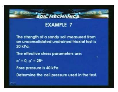
There is another example in which now we have the unconsolidated undrained triaxial strength, we have the c and phi dash values. This is nothing but the deviatoric stress these are the c dash and phi dash value, pore pressure is measured and we have to determine the cell pressure.
