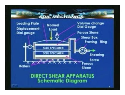
This upper portion is a part of the same container, the container is split into two halves and there is what is known as the yolk to which a proving ring can be attached, is fixed. And the soil specimen is kept in this container and the specimen again is kept in such a way that there is a small gap between the 2 parts of this container. So that the upper portion can be moved relative to the lower portion.
