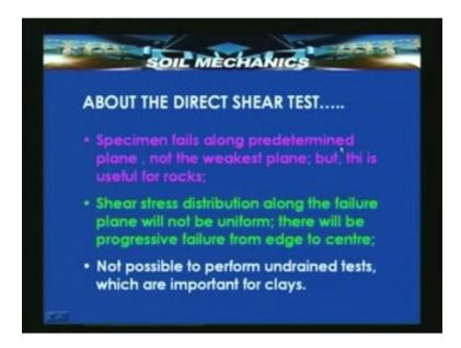
A specimen fails along a predetermined plane and not the weakest plane but in certain instances this is very useful. For example in rocks where there are predetermined joint planes which are already existing along which failure is likely to take place.
