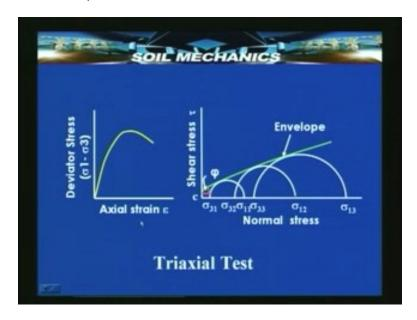
This is how the Mohr's diagram will look, if you do 2 or 3 test under the triaxial test and plot the sigma<sub>1</sub> sigma<sub>3</sub> plots and the Mohr's plot and as you apply the normal load the axial strain take
