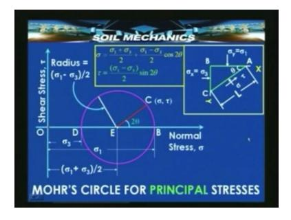
So once we know these 2 expressions we can compute sigma and tow from knowing the angle theta. So looking at this slide we can see that there is a minor different between general set of stresses and principle set of stresses.
