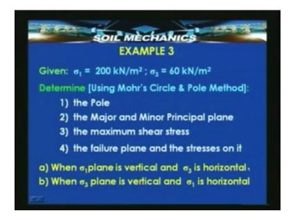
Again using the Mohr's circle and pole method determine first the pole then the major and minor principle planes, the maximum shear stress and the failure plane and the stresses on the failure plane. Under two conditions, one when sigma<sub>1</sub> plane that is the major principle plane vertical and the minor principle is horizontal and case b when the major principle is horizontal.
