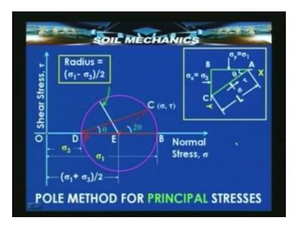
We have chosen the centre of the potential Mohr's circle; we have got the Mohr's circle and its radius. We have got the point C and how we have obtained is by choosing the point D which represents the state of stress corresponding to sigma<sub>3</sub>. That means the plane DC will have to be a line which is horizontal passing through the point D.
