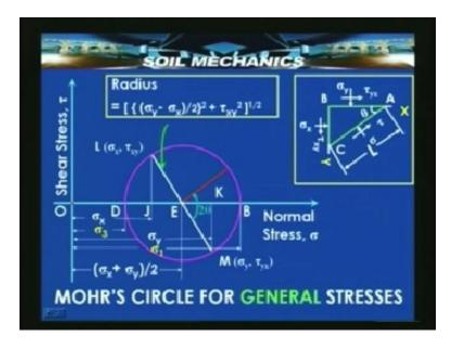
Now if we want the stress on the plane like CA, all that we need to do is to know the angle theta and then from this reference diameter draw a line at angle 2 theta taken in the anti-clockwise direction. And this red line typically represents the plane which we will get corresponding to the point C whose coordinates will be sigma and tow. So point C represents the stress level on the plane AC.
