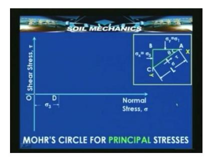
Obviously the center has to lie between D and B at its midpoint. So choose the origin E at the midpoint of the length DB. It will be equal to sigma<sub>1</sub> plus sigma<sub>3</sub> by 2. Plot the Mohr's circle with the radius as sigma<sub>1</sub>- sigma<sub>3</sub> by 2 then take an angle 2 theta with respect to the horizontal that is the line EB.
