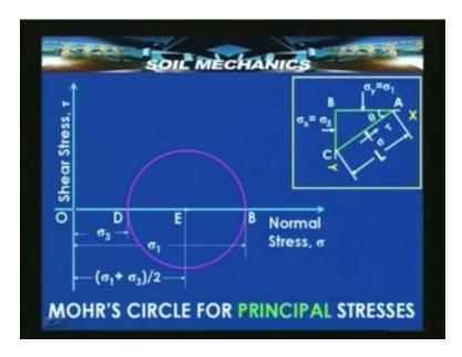
Get the red line, the coordinates of the points where the points intersect the Mohr's circle will be nothing but sigma and tow. So points C will represents the stress state on any arbitrary plane AC at angle theta and it can be shown that sigma will be equal to this, tow will be equal to sigma<sub>1</sub>-sigma<sub>3</sub> sin 2 theta.
