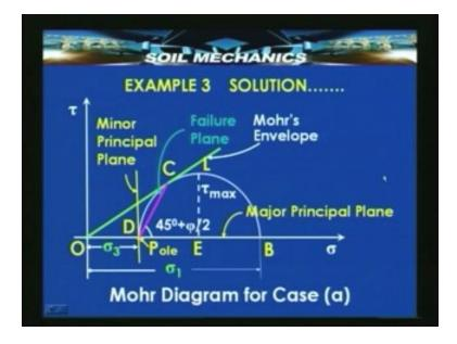
The solution is very simple as before plot the Mohr's circle and also after determining the pole P corresponding to the principle stress sigma<sub>1</sub>, get the failure plane corresponding to the point C and get the stresses.
