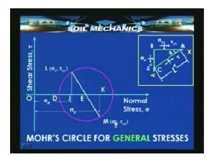
This is a circle, this circle intersects the x axis at point D and E, they have a significant as I briefly mentioned in 2, 3 slides ago. Point D has a least possible normal stress here and that's known as sigma<sub>3</sub>.
