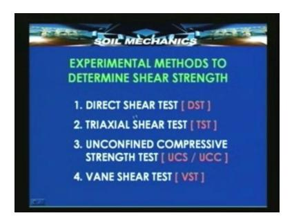
The commonly used methods for determining the shear strength are one direct shear stress DST for short, triaxial shear test TST, unconfined compressive strength test usually called as UCS or UCC, UCS standing for unconfined compressive strength, UCC standing for unconfined
