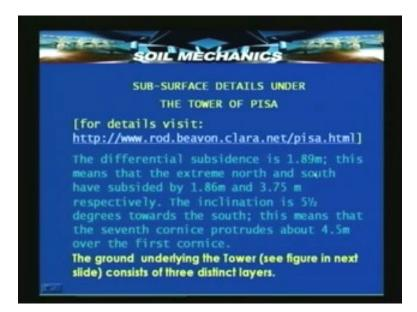
This means that the north and the south sides had a differential settlement amounting to the difference between 1.86 meters and 3.75 meters respectively. The tilt that took place because of this is 5 and a half degrees towards the north because the north as subsided more. This means that the seventh cornice, you know there are several levels, seventh cornice protrudes about 4.5 meters over the first cornice that is the amount of lateral movement that has arisen because of the settlement.
