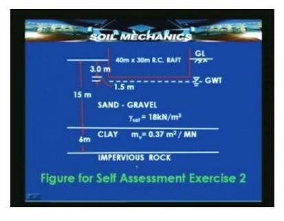
This is the illustration, again there is a clay layer above that is sand below that is impervious rock so this is an instances of single drainage. Then we have an exercise 3 in which we have to obtain this settlement at the end of several time periods 1, 5, 10 and 20 years. We can compute this as shown and the partial answers I have given already.
