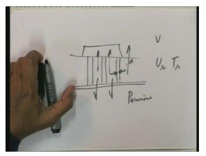
Similarly, analogously radial consolidation the degree of consolidation and the time can be expressed by identical equation. In place H we have 2 R. Now how does one get total consolidation which is given by this equation 1- U where U stands for the total consolidation is a product of 1-  $U_z$  and 1- $U_r$ .
