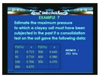
Now with this we also saw the example of how to the pre consolidation pressure, given the various e P values. The method is of course plot e long P graph and following the geometric construction which we saw in the earlier slide, you can calculate. Now you may work this out this example, you will find that a pre consolidation pressure as 293 kilo Pascal's.
