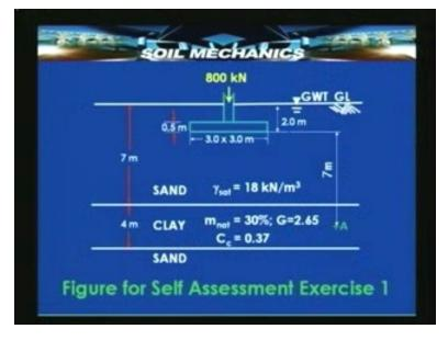
This is the illustration of fitting resting on a sand layer and a compressible clay layer followed again by a sand layer. So this is an instance of 2 way drainage.
