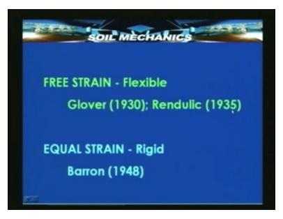
We saw that in order to solve this equation of radial consolidation, we could make either an assumption of free strains in the median or equal strains under the applied load due to the preload embankment. We generally use the equal strain technique which is a much simpler equation to handle and the solution to this was given Barron which I mentioned in the last class, in the last lecture.
