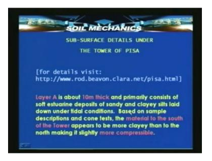
Now what is the reason for this settlement? You can see a lot of details about this including the details of the restoration of this in the website which I have listed here. The prime reason is there under sub surface condition there is a layer A which is 10 meters thick which is basically consisting of deposits of sandy and clayey silts.
