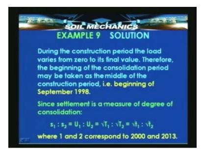
If beginning of September 98 is the point at which the load application takes place then it is given that 3 centimeter settlement takes place at the end of September 2000. So beginning of September 98 to end of September 2003, 3 centimeter settlement has taken place.
