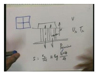
Next we know the value of  $C_c$  it is given and we have divided the layer into two, A and B. Now the total load of 1100 kilo Newtons is distributed over a foundation area of 49 square meters that means the loading intensity is 22.5 kilo Newton's per square meters and the depth upto point A or point B as the case may be or let us say  $h_1$  and  $h_2$ .
