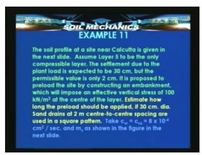
The example reads like this, the soil profile at a site near Calcutta is given in the next slide. Let us assume that the layer 5 in that profile is the only compressible layer. The settlement due to the load that is expected due to a structure there is 30 centimeters.
