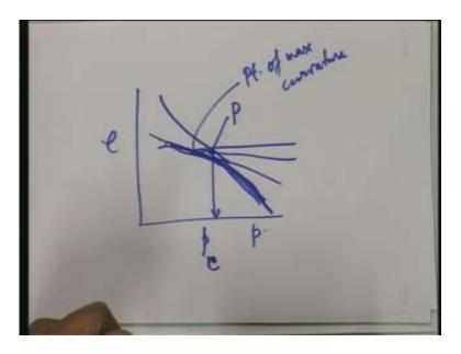
So if you plot this graph then particularly this is usually plotted to a log scale. So on a log scale if you plot this graph and estimate the pressure corresponding to this point where the bisector cuts the linear part of the curve you will get a value of 293 kilo Pascal for the pre consolidation pressure.
