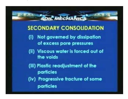
A mechanical way an example is compaction. During compaction some amount of water also goes out that which is adhering to solid particles do go out but basically this water which is viscous in nature is what is driven out during constant effective stress during the secondary consolidation process. And it is during this process of viscous water moving out that plastic adjustment or deformation of particle takes place and so the third point is plastic readjustment of the particles.
