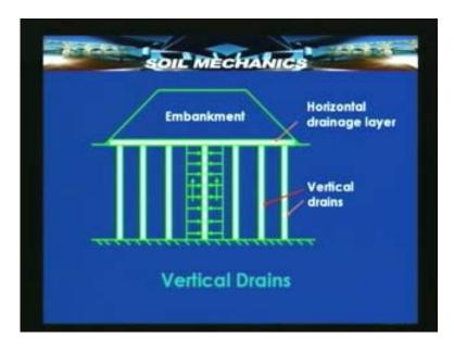
Take look at this slide. We have here as I already explained in the last lecture an embankment sitting over soil surface. There is a compressible soil layer here and what you see here driven or placed or erected in this compressible soil layer are vertical drains. These are nothing but vertical bore holes which are filled with some highly pervious materials like sand and on top again there is an embankment below which, at the base of which we have a horizontal drainage layer that is
