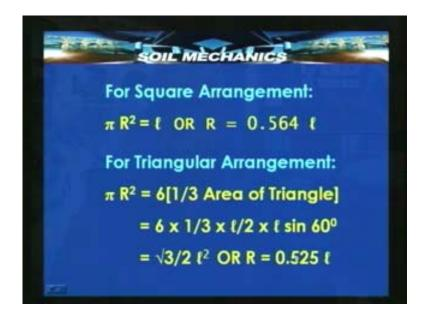
On the other hand if you take the triangular arrangement each cylindrical drain will have to cater to one third of the neighboring triangular triangle and therefore totally 6 triangles of this area should be equal to pi R square. So from here that we will find 6 into 1 by 3 into 1 upon 2 into 1 upon sine 60 which is nothing but the area of the triangle. See here 1 upon 2 into 1 this angle is 60 degree because this is a an equilateral triangular arrangement and therefore this length will be
