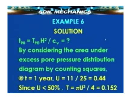
So let us see by considering the area under the excess pore pressure distribution diagram in terms of the number of squares into which we have divided the diagram. We can find out at t equal to one year to which this figure corresponds, what part of this area it is under this curve, out of the total area? That is what is the area occupied by this curve as a fraction of the total area occupied by the u equal to the  $u_i$  curve.
