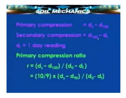
So the dial reading is  $d_s$  to  $d_{100}$  that represents the primary consolidation where as  $d_{100}$  to  $d_f$  represents the secondary compression and if  $d_f$  usually is taken in after about a day after this 100% consolidation can be considered to be over. That is after the dial gauge readings have become practically stable, constant we take that has the point
