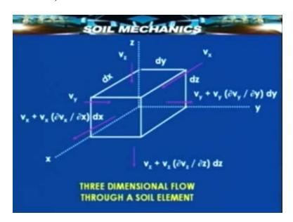
So now you should take y direction,  $V_y$  is the in flow  $V_y$  plus this into dy becomes the outflow and for the z direction this is in flow and this is the outflow (Refer Slide Time: 37:33). So now the flow equation very similar to the one dimensional consolidation flow will lead to once again an expression in which there is a volumetric compression and the rate at which that volumetric compression takes place will be or can be related to the total
