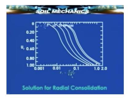
So we can get  $T_r$  as a function of this R for equal strain condition and corresponding Ur using the so called the Barron's equation and this is a graph which represents this, we can also use a look up table for this purpose. So in this lecture we had seen a couple of examples then we have discussed the secondary consolidation phenomenon and we have seen the importance of radial consolidation. In the next lecture we will continue and see some more examples.
