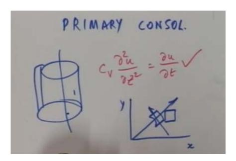
So if I add to this the z dimension then it becomes a truly three dimensional phenomenon. What this means is our three dimensional problem in terms of polar coordinates can be treated as a vertical compression problem corresponding to the same z coordinate as in the Cartesian system plus a consolidation which is now a function of the radial direction which is a function of the radial coordinate r.
