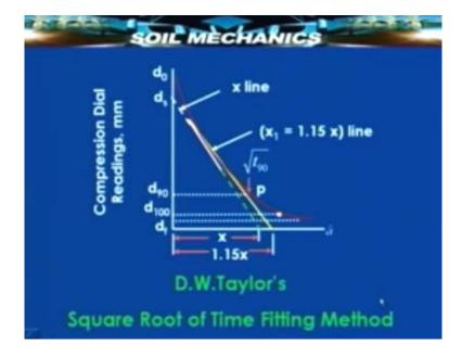
The dial gauge reading corresponding to that state is ds and now starts the compression arising out of the hydrodynamic lag and it goes on until we reach the  $d_{90}$  point. If we allow this phenomenon to continue we will end up with after a few days say some times 24 hours some times 48 hours, we will find that the dial gauge readings reach a very
