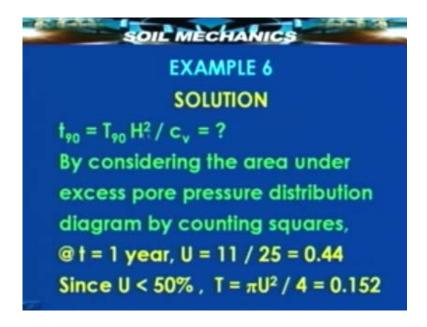
We know that the system is a double draining system and the thickness of the clay layer if we know then we can calculate  $C_v$ . What we actually need is the time corresponding to
