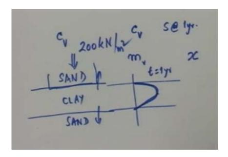
So let us take a look at the pore pressure distribution. This is a curve showing the pore pressure distribution. This is depth, this is the excess hydrostatic pressure and this is a curve of distribution.
