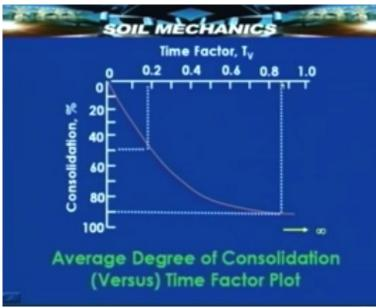
And that's shown here for 90% we have 0.848 and for 50%, 0.97. Here is again the average degree of consolidation over the entire depth and once again you find that at time
