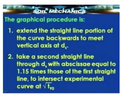
So if you have the initial dial gauge reading  $d_0$ , first you have to work out the corrected zero dial reading after accounting for gas expansion and so on. Because that's the point where the straight line part of the curve will cut the y axis. So  $d_0$ - $d_s$  is the initial
