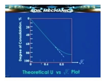
Where as now we find that once it is plotted against root of time, it has become almost a straight line. Now this straight line is the basis for comparing this curve now with a curve obtained from typical oedometer test, a curve of dial gauge reading versus root of time in the method. So the initial part of the theoretical U versus root of  $T_{\nu}$  curve is found to be linear, is linear up to 60% consolidation.
