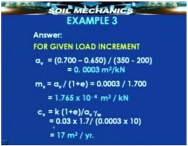
Let us take another example. A 6 meter thick clay layer is subjected to a load of 60 kilo Newton per meter square. One year after loading the average consolidation u is found to
