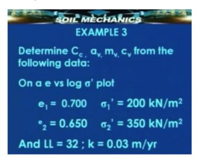
So answers are  $c_c$  will be equal to the change in void ratio divided by logarithm of the ratio of stress that is 0.206.
