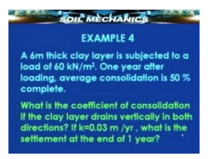
What is asked is the coefficient consolidation assuming one dimensional consolidation and if k=0.03 what is the settlement at the end of one year? The settlement that will really take place here will depend upon the final void ratio. So at this point of time, interested in the settlement corresponding to a particular time rather than the total settlement. And that's why we need the coefficient of consolidation here.
