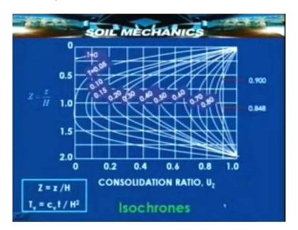
In that expression for  $U_z$  we had non dimensional depth z by H and the non dimensional time factor  $T_v$ . So suppose we substitute different values of T, T =0, 0.05, 0.1 and so on up to 0.9. Then we find that at different values of z by H we will get different  $U_z$  values and this is how the  $U_z$  values will vary, these are known as isochrones indicate meaning that these are the values of  $U_z$  corresponding to constant time or constant time factor.
