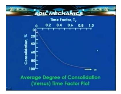
Suppose we know how the average consolidation over the entire depth can be determined. Then we will find that this average consolidation varies with time as shown in this diagram that is it goes on increasing with time and ultimately at time t equal to infinity it's completed that is 100% degree of consolidation is achieved.
