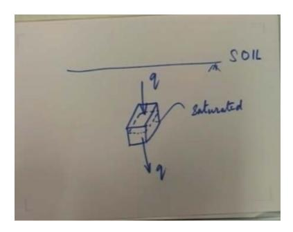
Suppose there is an in flow which can be represented as a  $v_z$  where  $v_z$  is the velocity. Velocity as we know is nothing but flow per unit time and in this case if we consider unit area then  $v_z$  will be nothing but velocity is nothing but flow per unit area per unit time and if the area is of finite dimensions delta x delta y as shown here where x y z axis are also shown. Then the inflow and out flow because they are going to be different in this medium.
