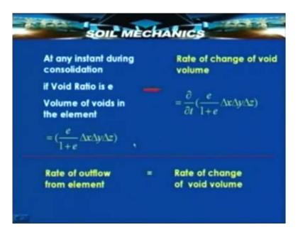
Now as the flow takes place from inside the element to the outside, these volume decreases. So the volumetric change in unit time that is the rate of change of volume which is nothing but the rate at which the compression takes place is going to be the derivative of this volume of voids with respect to time and that's what is the rate of change of voids.
