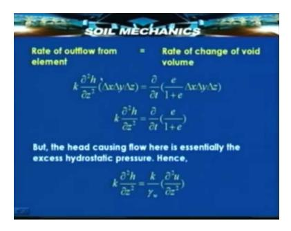
So this del square h by del z square can be written as u upon  $gamma_w$  and so we will have k upon  $gamma_w$  del square u by del z square where u now is the excess hydrostatic pressure. This must now be equal to del by del t of e upon 1+ e this, so let us equate them. If you equate, this (Refer Slide Time: 26:35) is what you get but before equating let us see what this del by del t e upon 1+ e is. We have just now stated that 1 upon 1+ e is the unchanging constant volume of the solids.
