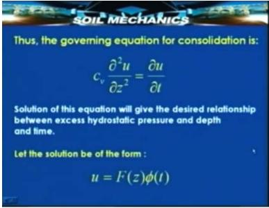
And suppose following that we express the excess hydrostatic pressure as a product of two independent functions. One a function of only z another a function of only t then
