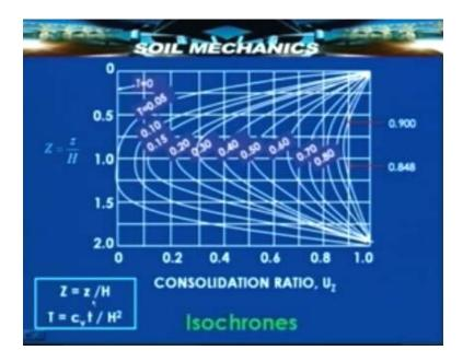
Now since the degree of consolidation varies with depth we preferably need to have a parameter which gives us an average degree of consolidation over the entire depth of the clay layer and we will be seeing how that is defined.
