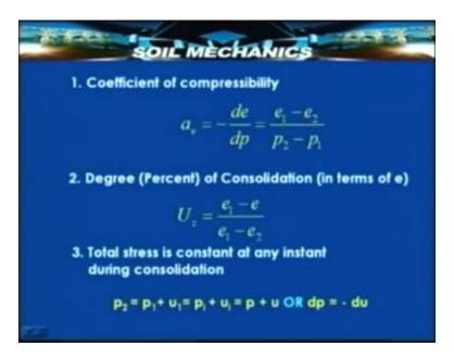
So that we can get the value of degree of consolidation at any point of time. So for this purpose suppose we take advantage of the fact, the total stress is always equal to the pore pressure plus the effective stress then p<sub>2</sub> at any instant, at any second instant you can say will be equal to the effective stress in the first instant plus the excess hydrostatic pressure in the first instant.
