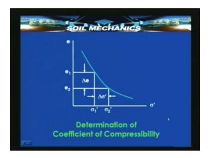
These 2 parameters are particularly useful to us for computing the time rate of compression. Because these ep curve which is non linear has values of  $a_{\rm v}$  and  $m_{\rm v}$  which go on changing with time as the stress changes.
