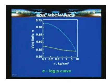
For example that parameter is known as the coefficient of compressibility and that's equal to the void ratio change divided by not the logarithm of stress change but the stress change itself. Now we also have another parameter known as the coefficient of volume decrease or volume change or volume compressibility which is nothing but the change in void ratio per unit void ratio divided by delta sigma dash that is  $a_v$  upon  $1+e_0$ .
