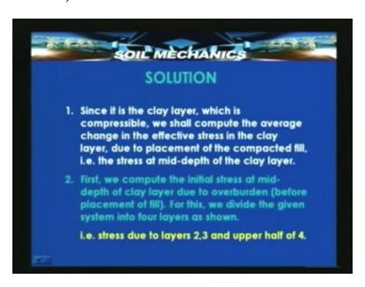
So for all practical purposes we will assume that the clay layer is homogenous and an average value of stress change or void ratio can be obtained by simply considering a point at mid depth of this clay layer.
