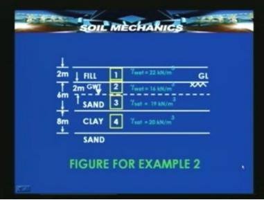
We need to make assumptions like this, from point of view of drainage. The reason why we have taken sand layers above and sand layers below is we are going to assume one
