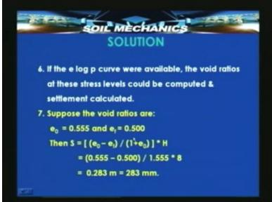
How ever we can also compute this settlement in terms of the stress changes that is by using a formula which computes the settlement in terms of the relationship between void
