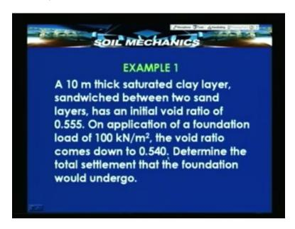
Suppose we take one simple example. A 10 meter thick saturated clay layer sandwiched between 2 sand layers has an initial ratio of 0.555, a final void ratio of 0.540 and a load
