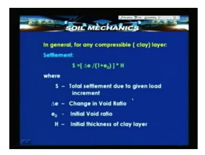
So s is the total settlement due to any given load increment, delta e is the change in void ratio,  $e_0$  is the initial void ratio and capital H is the initial thickness of the clay layer. This is how we compute the settlement in terms of the void ratios.
