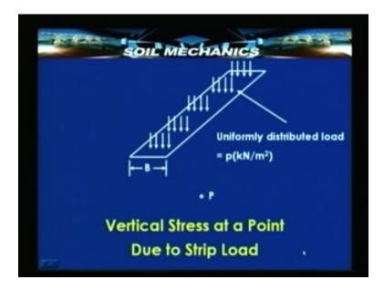
We shall see how to compute the stress below a strip load. Let us take a look at this slide. The strip load here is defined by a width B and a very long length. The length is very large and that is why no specific length is mentioned here. For all practical purposes it can be taken as infinitely long compared to B. And now if you want the stress due to this load at point P then we can proceed using the line load formula. (Refer Slide Time 19:18)
