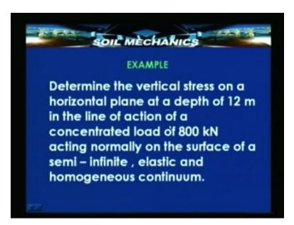
Determine the vertical stress on a horizontal plane at a depth of 12 meters due to a concentrated load 800 kilo Newtons in an elastic medium. So the solution would be find out r by z, it so happens that if r/z is zero  $I_f$  is 0.47745. This is happening because we
