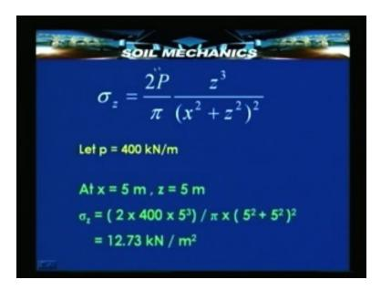
Now comes the importance of the use of sigma z computation by the principle of super position. Take for example two concentrated loads  $P_1$  and  $P_2$  and any point A in the medium  $P_1$  is 400 kilo Newton per meter. This is a line load actually 400 kilo Newton per meter in a direction like this and  $P_2$  1000 kilo Newton per meter again a line load along this.
