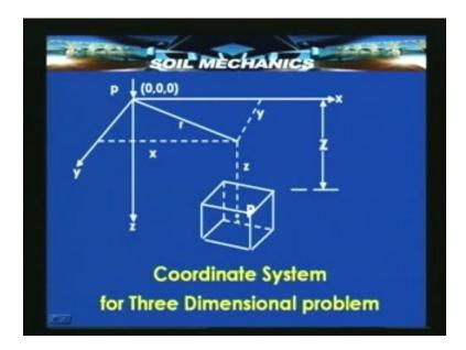
So this is the element which we shall be analyzing to find out what is the stress in the element. And this is the coordinate system that we shall be using and this is the load P which is known as the point are the concentrated load, due to which we are interested in finding out what this stress at point P. We were taking a look at the fundamentals of the theory of elasticity yesterday. The theory of elasticity assumes 4 or 5 major tenants. Number one, it says that the material is in equilibrium.
