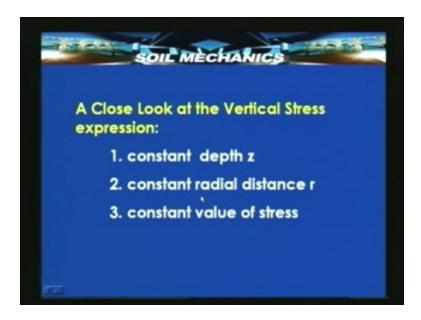
I am taking a constant value of z and at a constant value of z as r increases, how the influence factor varies and how the stress varies? Suppose we start with r equal to zero, at r equal to zero the influence factor can be computed from here to be equal to 0.4775. And as I mentioned while showing the previous slide at r = 0, the maximum stress occurs. So here this shows that r = 0, the influence factor is 0.4775 and the maximum stress that occurs at r = 0 is P upon z square into 0.4775.
