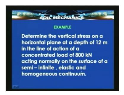
Applying our expression for sigma z, which is P by z square into the influence coefficient. At r/z = 0 we find that influence coefficient is 0.47745 which means that the stress sigma z is nothing but 2.653 kilo Newton per meter square. You see how simple the problem of stress computation has become. This has helped us to find out the stress at r/z = 0, that is at r = 0 and z = 0, at that top surface. This is the maximum value of the stress due to the applied load in this particular problem.
