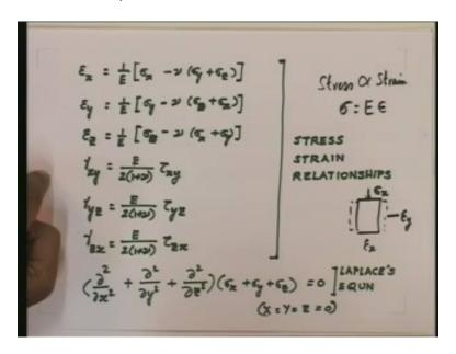
And so the stress strain equation or rather the strain stress equation or relationship for epsilon x in terms of the three unknown stresses will be like this. We have to appreciate the fact that we have succeeded in creating an equation based on theory of elasticity in which we have not introduced any new unknown.
