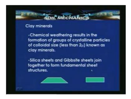
The three basic clay minerals are Kaolinite, Illite and Montmorillonite. Kaolinite is generally prevalent in sedimentary and residual soils. Illite is common in stiff clays and shales as well as in post glacial marine and lacustrine soft clay and silt deposits. Montmorillonite is the third mineral; it is the dominant clay mineral in some clays and shales and in some residual soils derived from volcanic ash like Bentonite. Other minerals form Halloysite, Chlorite, Attapulgite and Allophane.
