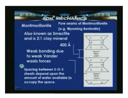
The nature of bonding in Montmorillonite elementary layer can be seen here, where alumina sheet get sandwiched with the help of silicate sheet and another silicate sheet at the bottom. This is represented here in this slide: alumina sheet or GIBBSITE sheet and silicate sheet at the top and silicate sheet at the bottom.
