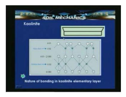
A Kaolinite crystal or particle consists of a stack of several layers of the basic 7.2 Angstrom thick layers. Here a typical Kaolinite particle has a length equivalent to 1000 to 20,000 Angstrom units and its thickness is 100 to 1000 Angstrom units. This Kaolinite particle is formed typically by 70 to 100 elementary layers. This forms strong hydrogen bonds between the hydroxyls of the GIBBSITE sheet and oxygen of the silicate sheet.
