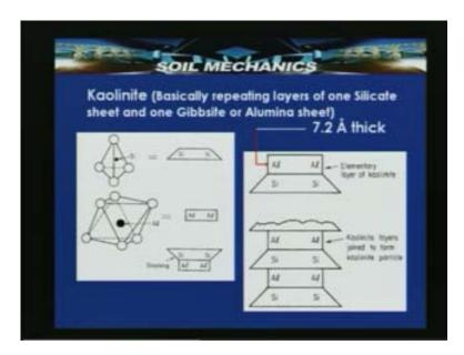
Here the nature of bonding in Kaolinite elementary layer is shown and how the silicate sheet and alumina sheet are attached is also shown in this slide. This is an alumina sheet and this is the silicate sheet.
