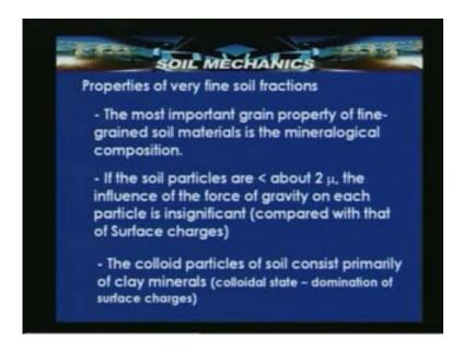
Before defining clay mineral, let us define a mineral. A mineral is a naturally occurring chemical element or compound formed by a geologic process. Classification of minerals based on the nature and arrangements of atoms can be in the following ways: Carbonates, Phosphates, Oxides and Silicates.
