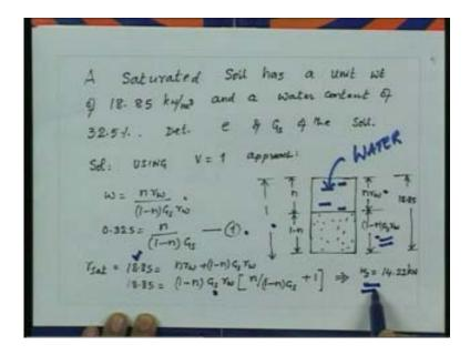
Now we can solve by using this unit volume approach the void ratio as 0.463 and volume of solids is equal to 1 minus 0.463 that is void ratio is equal to 0.86 where e is equal to n
