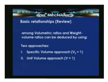
In this lecture let us look into the methodology of the unit volume approach. In the unit volume approach, the total volume v is set as 1 as the phase diagram method requires certain quantity of soil to be specified. So here the total volume is set as 1. Basically the Porosity n is used in place of void ratio here. This approach is used when no weights or volumes are given in the problem statement, so one can select depending upon the problem statement.
