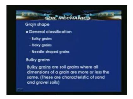
Now let us look here, the source of this bulky grains are mechanical breakdown of parent rocks. During their transportation by wind or water, the sharp edges of the grains may get worn out and the grains may become rounded. For example gravels which are found along the river beds like river gravels or wind blown sands like dune sands the grain
