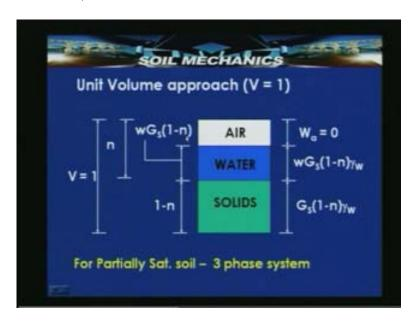
Let us look into the deduction of this particular figure for a partially saturated soil 3-phase system. We know n Porosity is equal to (volume of voids to total volume) with V is equal to 1 in unit volume approach, n is equal to  $V_v$  now the volume of voids is set as n. Then void ratio is equal to (ratio of volume of voids to volume of solids), it is nothing but n by (1 minus n).
