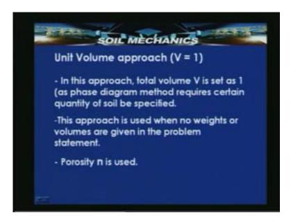
Now let us consider for the unit volume approach V is equal to 1 and for a partially saturated soil a 3-phase system where there are solids, water and air. On the right hand
