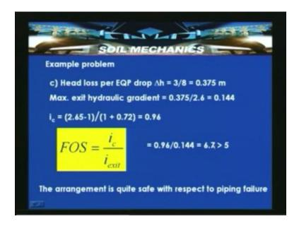
So by knowing the critical hydraulic gradient and particularly the exit gradient, we can calculate the factor of safety against piping or heaving failure. And here the critical hydraulic gradient happens to be 0.96 divided by 0.144 which is around 6.7. So this actually happens to be more than 5. So this indicates that the arrangement whatever is been shown with particular dimensions is quite safe with respect to piping failure.
