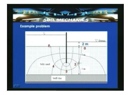
This is the first equipotential lines zero that is equipotential drops, second, third, four so on to eight equipotential drops which are shown. Schematically 1, 2, 3 and around 2.5 flow channels are shown here.
