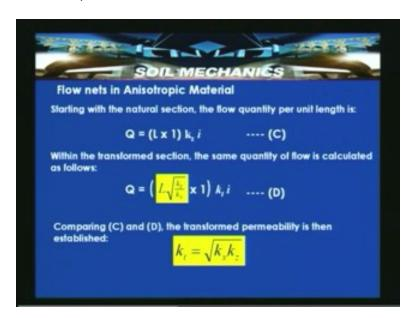
Now starting with the natural section that is on the left hand side in the previous slide. The flow quantity per unit length can be written as  $Q = (L \times 1)$  that is area over which the flow is occurring into  $k_z$  that is the permeability and i is the hydraulic gradient with which
