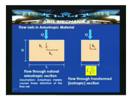
So this length is taken as L into root over  $k_z$  by  $k_x$ . Even with this transformation or whatever we are doing we should see that the laplacian equation is satisfied. So here the length is L into root over  $k_z$  by  $k_x$  and which is being small because we have already discussed that  $k_x$  is always more than  $k_z$ . That is our assumption that the horizontal permeability is more than vertical permeability.
