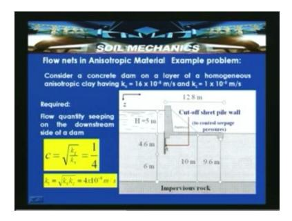
So x is the horizontal direction and z is the vertical direction. The length from here to here is 12.8 meters and 5 meters is the head which is available on the upstream side and the depth of the cut of sheet pile wall is 4.6 meters and the tip is 6 meters above this impervious rock under consideration (Refer Slide Time: 23:36). So from the flow net what we require is the flow quantity seeping on the downstream side of a dam that is seeping through the soil.
