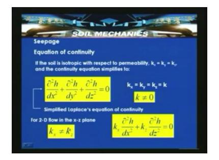
So for two dimensional flow in x z plane, if the  $k_x$  is not equivalent to  $k_z$  say an anisotropic, as far as two dimensional flow is concerned then we can say that  $k_x$  into dow square h by dow x square +  $k_z$  into dow square h by dow z square is equal to zero. So here we can say that for a dimensional flow in x z plane the  $k_x$  is not equivalent to  $k_z$ .
