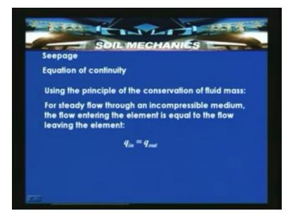
So by substituting from the previous discussion and by simplifying we will get an equation  $q_x$  which is  $q_x + q_y + q_z = q_x + dq_x + q_y + dq_y + q_z + dq_z$ . The simplification of that yields  $k_x$  into dow square h by dow x square +  $k_y$  into dow square h by dow y square +  $k_z$
