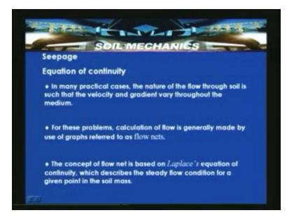
So coming to the seepage and equation of continuity, in many practical cases the nature of the flow through soil is such that velocity and gradient vary throughout the medium. So for these problems calculation of flow is generally made by the use of a graphical procedure called flow net methods. So this flow net method is nothing but the solution of the equation of continuity which we are going to derive very shortly.
