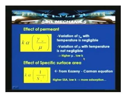
That means depending upon the type of mineral for example kaolinite, Montmorillonite and elite. The kaolinite has got lower specific surface area compared to Montmorillonite. So that means the soils which are having Montmorillonite can have low permeability compared to soils which are having kaolinite. Similarly the quartz which is having very low specific surface area exhibits very high permeability with this particular relationship.
