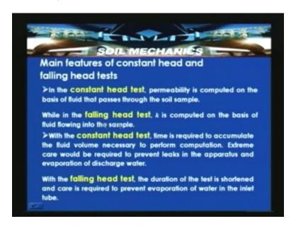
So main features are the major differences between constant head test and falling head test, they can be classified like this. In the constant head test permeability is computed on the basis of the fluid that passes through the soil samples. While in the falling head test, k is the coefficient of permeability is computed on the basis of fluid flowing into the sample. So here the amount of discharge that is the flow which is taking place into the sample.
