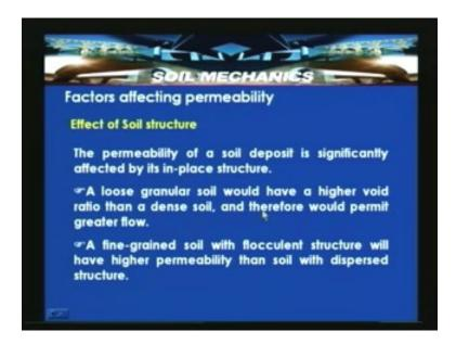
Another important parameter which influences the permeability is the soil structure. The permeability of a soil deposit is significantly affected by its in-place soil structure that is in-situ soil structure. A loose granular soil would have a higher void ratio than a dense soil and therefore would permit greater flow. That is the reason why we have discussed
