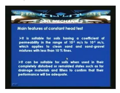
Let us look the main feature of the constant head test. It is suitable for soils having a coefficient of permeability in the range of 10 to the power of minus 2 to 10 to the power of minus 5 meter per seconds.
