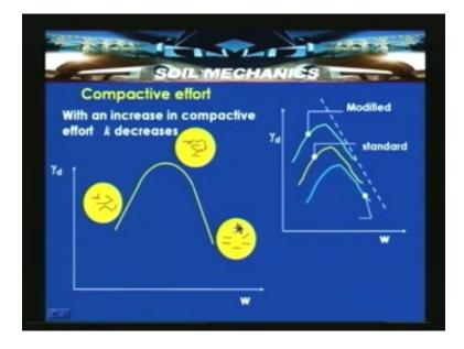
So if you recall the variation of gamma d versus water content can be obtained like this. This is for the reduced compaction and this is for standard proctor compaction and this for modified proctor compaction. With an increase in compaction energy there will be decrease in the opto moisture content, increase in the dry unit weight. And this line is the
