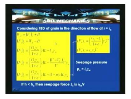
So considering the free body diagram of the grain in the direction of the flow at  $i = i_c$ . So we will derive for  $i=i_c$  an expression for seepage force. Then we will try to deduce a
