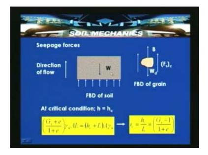
So  $h_c$  here is defined as a critical head. So  $G_s+$  e by 1+e gamma w AL indicates something like the saturated unit weight of a soil mass. The expression we know for a two phase system under saturated conditions, gamma sat can be written as  $G_s+$  e gamma w by 1+e, A is the area of the cross section over which the flow is taking place, L is the length of the sample.
