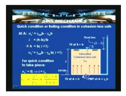
Now let us consider in this slide a thickness of a soil bed which is undergoing upward flow is b and h- b is the head loss taking place between these two levels. And total head at point B is small b and total head at A is h. So the difference is nothing but h - b, that is the head loss. Hydraulic gradient here i= h- b by b.
