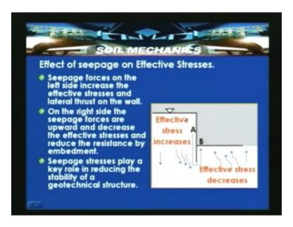
So seepage forces on the left hand side increase the effective stress and the lateral thrust on the wall. So with an increase in the effective stress it exerts also and in lateral thrust on the wall. On the right hand side the seepage forces act in the upward direction, because the flow is in the upward direction and decreases the effective stresses and
