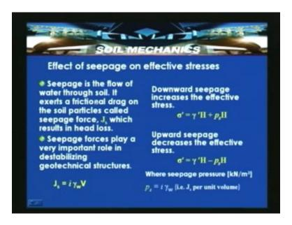
And which results in head loss because of the mobilization of the seepage forces it results in that head loss which is actually driving the flow. And seepage force plays a very important role in destabilizing geotechnical structures, like we discuss it just now. Particularly the seepage process play a very important role in destabilizing geotechnical
