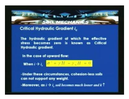
What is this critical hydraulic gradient? We have defined that the hydraulic gradient at which the effective stress become zero is called the critical hydraulic gradient. That means if you maintain particularly for upward flow condition, if you increase the head constantly, at a certain head it reaches the critical head where it can lead to a critical hydraulic gradient and lead to an effective stress zero in the soil. That means the soil loses all its supporting capacity to support the load.
