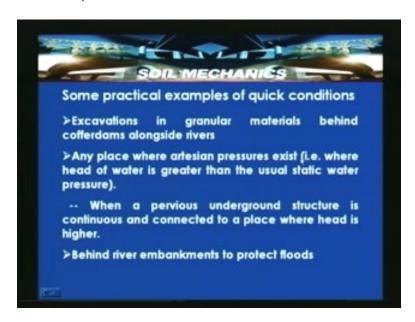
Any place where artesian pressure exist that is where the head of the water is greater than the usual static water pressure. So when a pervious underground structure is continuous and connected to a place where the head is higher. So the artesian condition means the definition can be defined like this, when a pervious underground structure is continuous and connected to a place where the head is higher. Then it can be subjected to artesian condition then flow can be upward.
